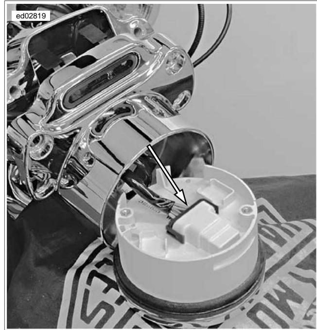
**Figure 4-64. Speedometer Connector [39] (Typical)**
