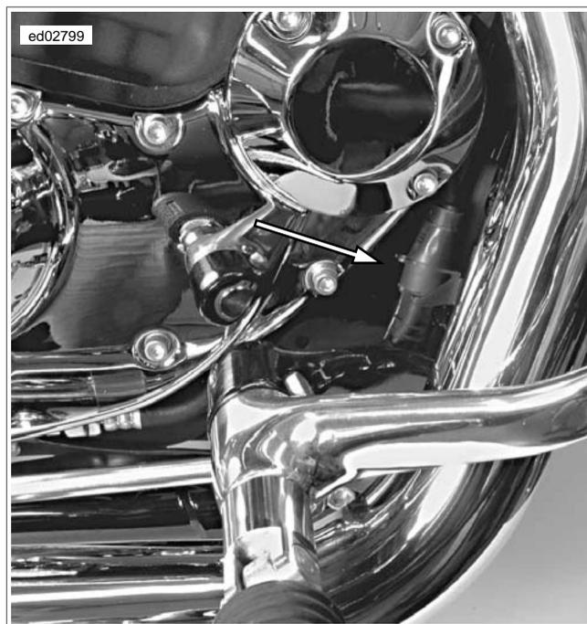
Figure 1-13. Stator Connector [46]
