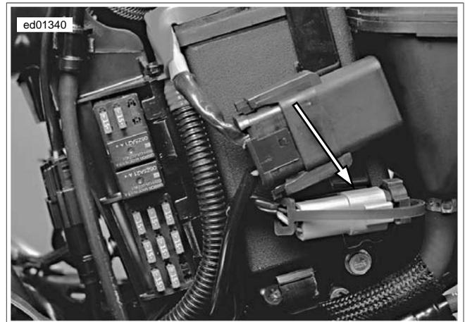
**Figure 2-21. Data Link Connector [91A] (Behind Left Side Cover)**
