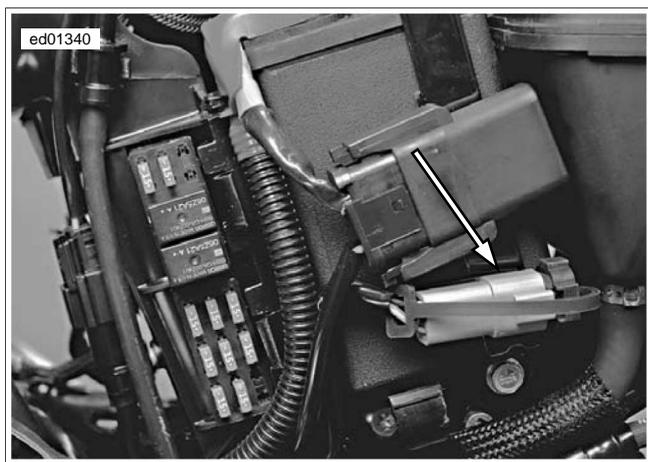
**Figure 4-19. Data Link Connector [91A]**
