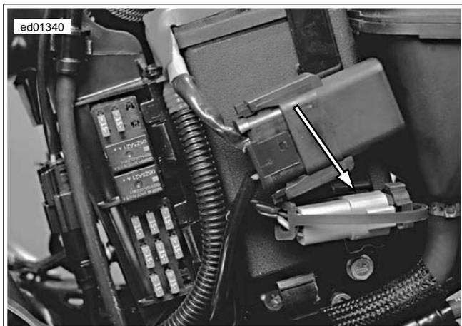
**Figure 2-16. Data Link Connector [91A] (Behind Left Side Cover)**
