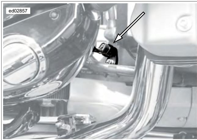
**Figure 4-48. Vehicle Speed Sensor and Connector**
