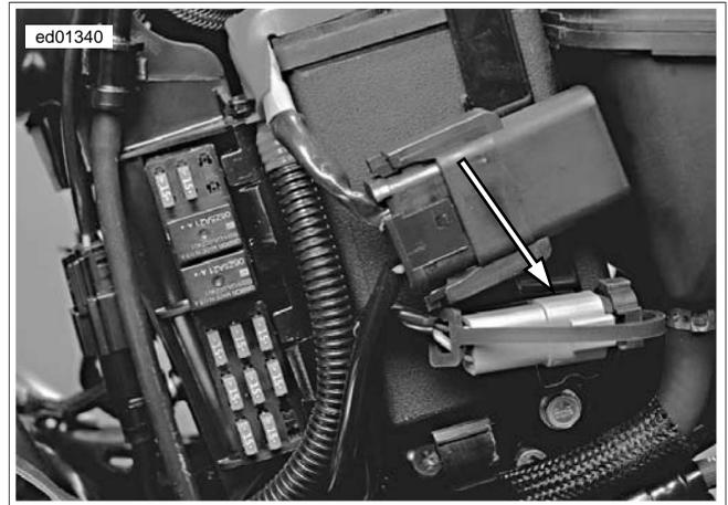
Figure 3-31. Data Link Connector [91A]
