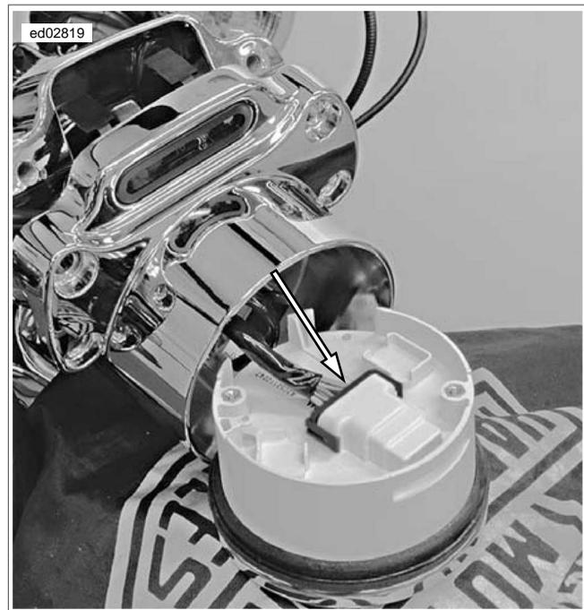
**Figure 2-18. Speedometer Connector [39] (Typical)**
