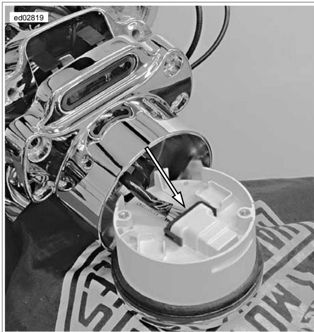
**Figure 2-12. Speedometer Connector [39] (Typical)**
