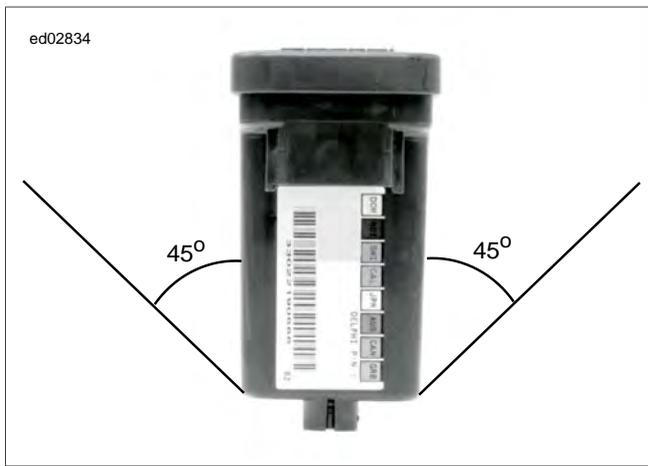
**Figure 3-22. Tilting: TSM/HFSM**
