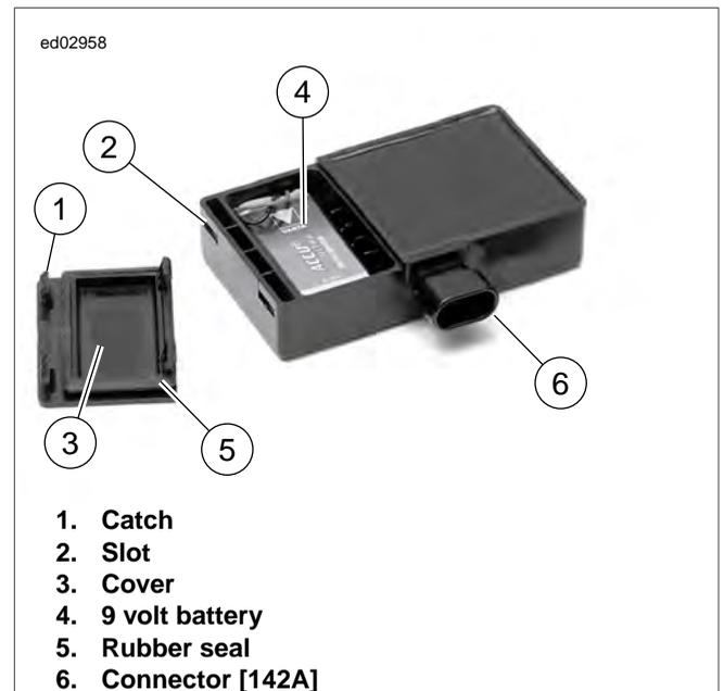
Figure E-32. Siren Battery Compartment (Late Style Siren)
