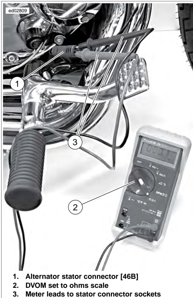
1. Alternator stator connector [46B]
