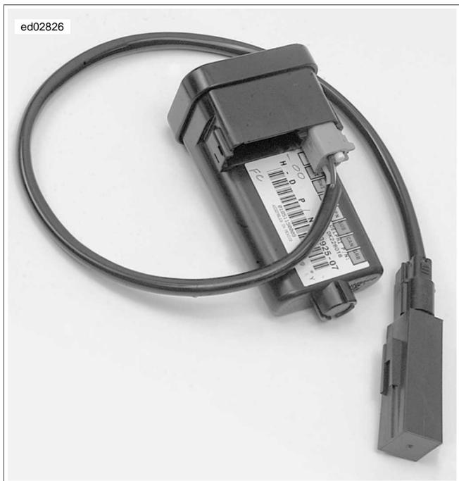
Figure 3-18. HFSM and Antenna
