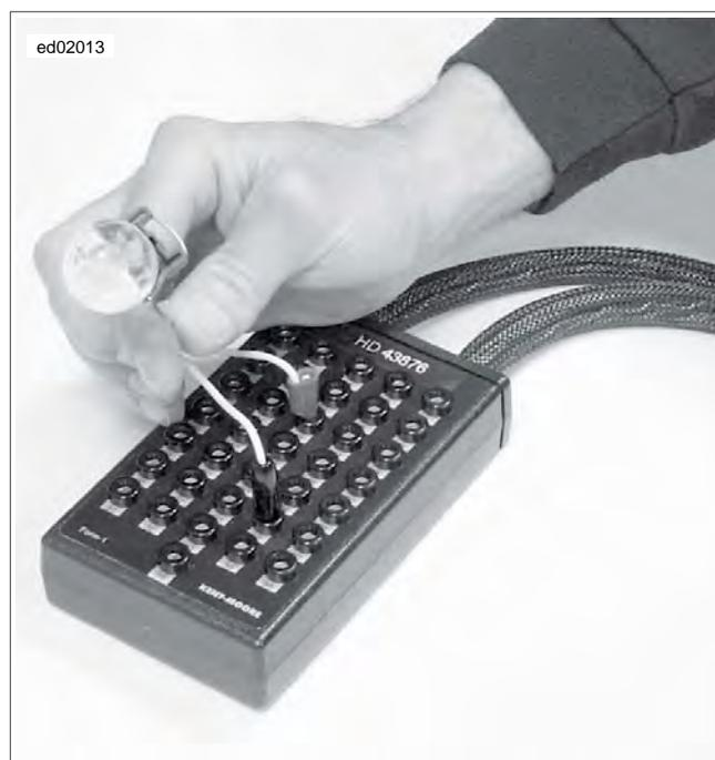
**Figure 4-15. Ignition Coil Circuit Test**
