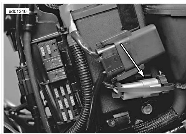
**Figure 4-52. Data Link Connector [91A]**
