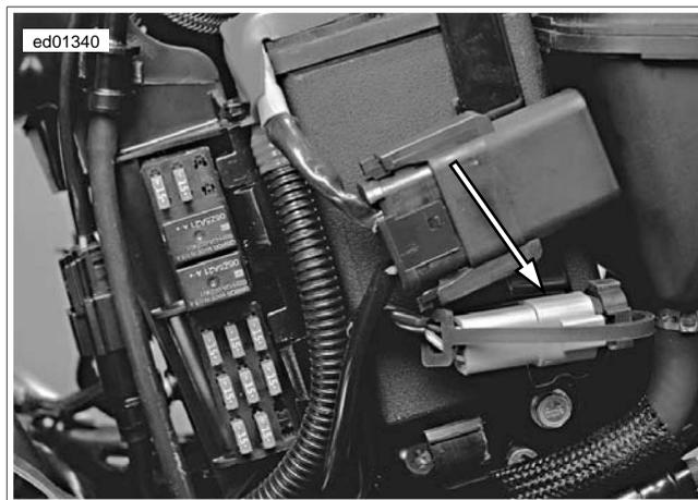
**Figure E-28. Data Link Connector [91A]**
