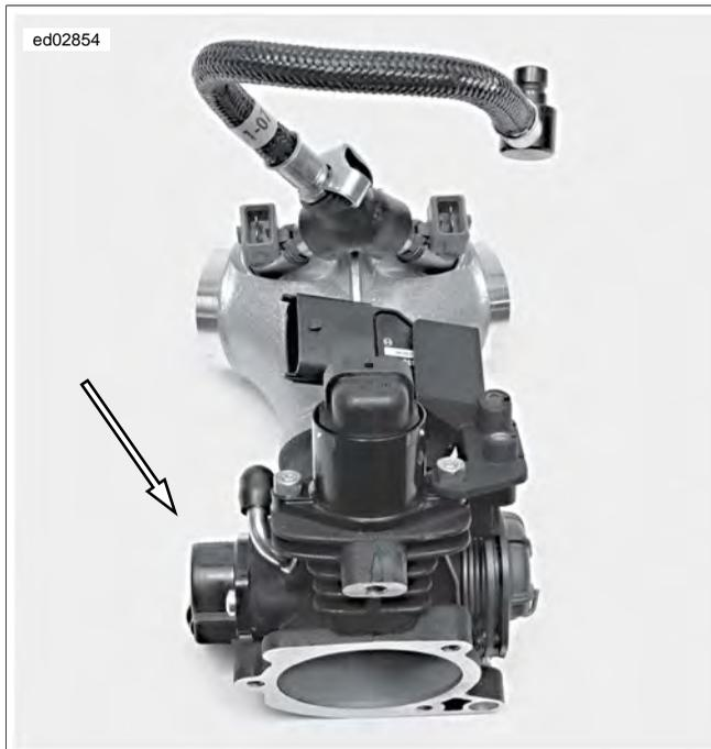
**Figure 4-40. Throttle Position (TP) Sensor Location**
