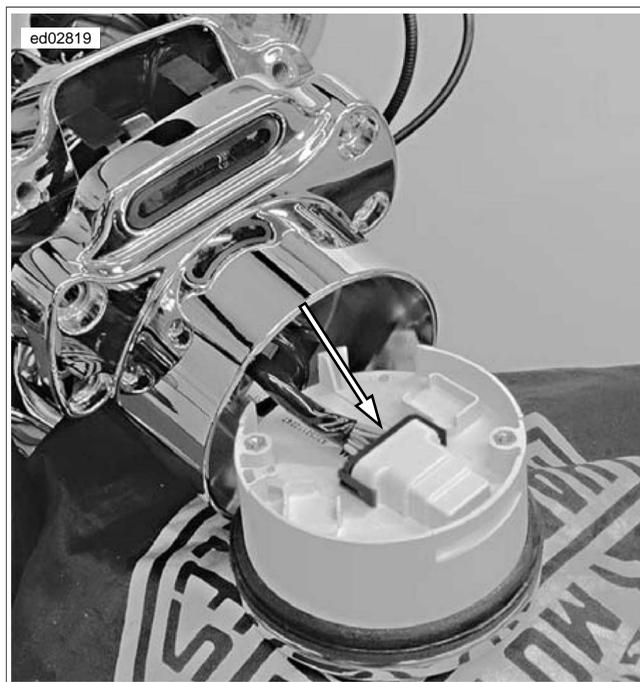
Figure 2-9. Speedometer Connector [39] (Typical)
