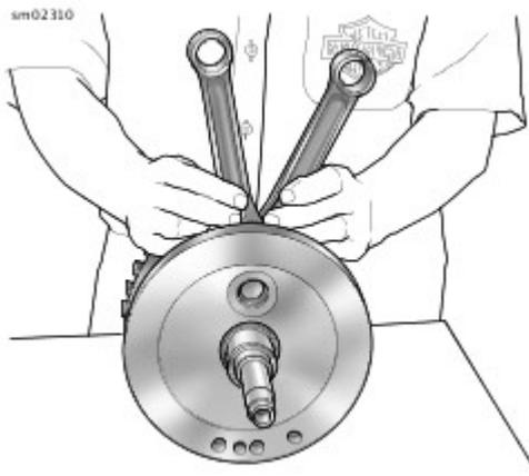
Figure 1. Connecting Rod Bearing Clearance
