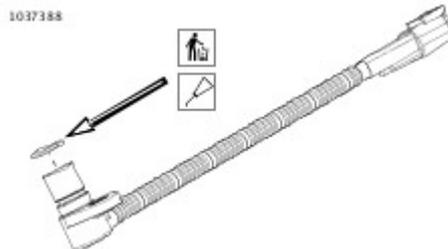
Figure 2. CKP Sensor Assembly
