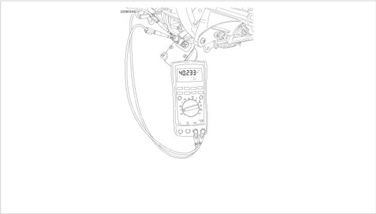
Figure 5. Check Stator AC Voltage Output (Typical)
