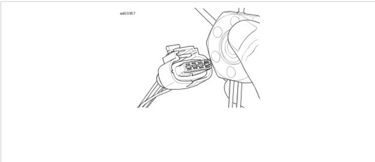
Figure 1. Terminal Removal: Bosch Compact 1.1M Connector
