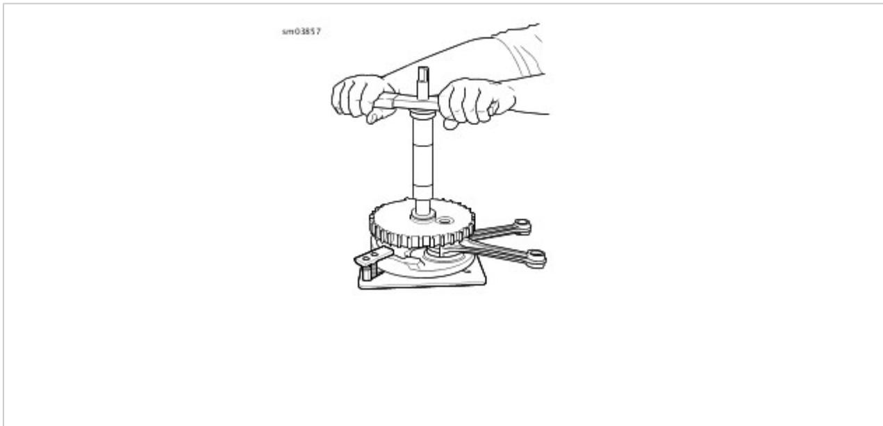
Figure 3. Press Inner Race onto Sprocket Shaft: Operation
