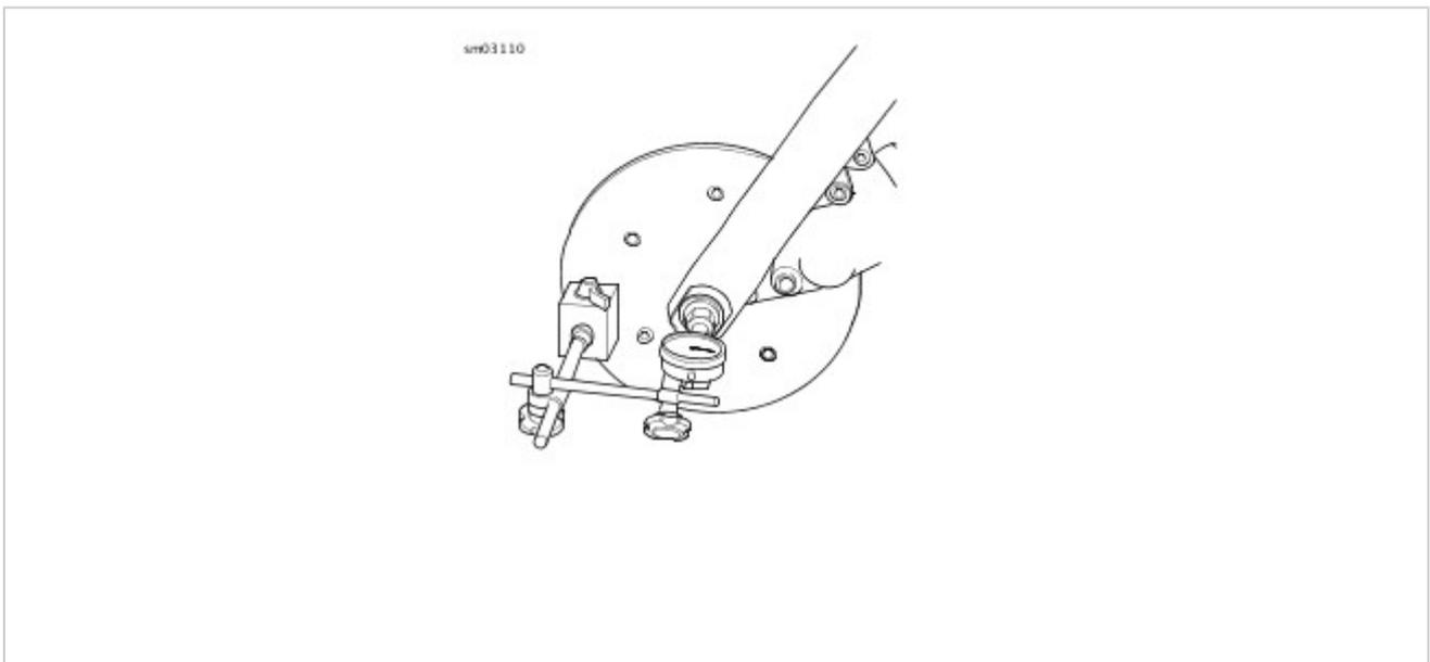
Figure 1. Measuring Lateral End Play (Front Wheel) (Typical)
