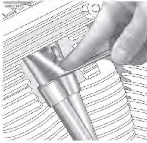
Figure 1. Install Spring Cap Retainers
