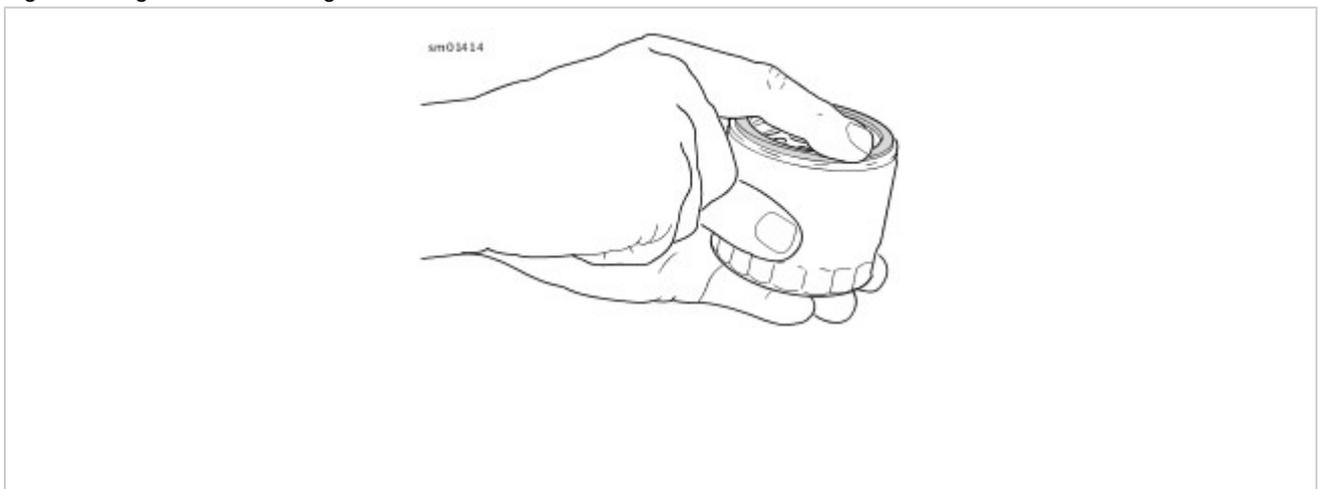
Figure 2. Lubricating New Oil Filter Gasket
