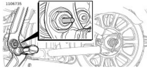
Figure 4. Rear Fork Pivot Shaft Alignment Rod
