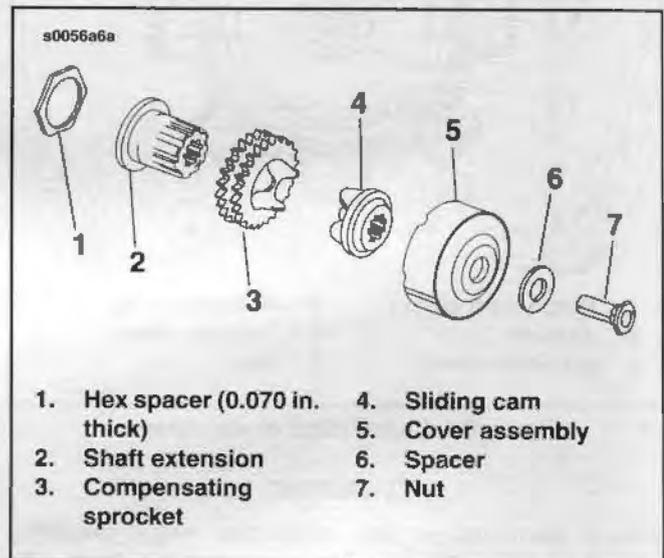
Figure 6-7. Compensating Sprocket
