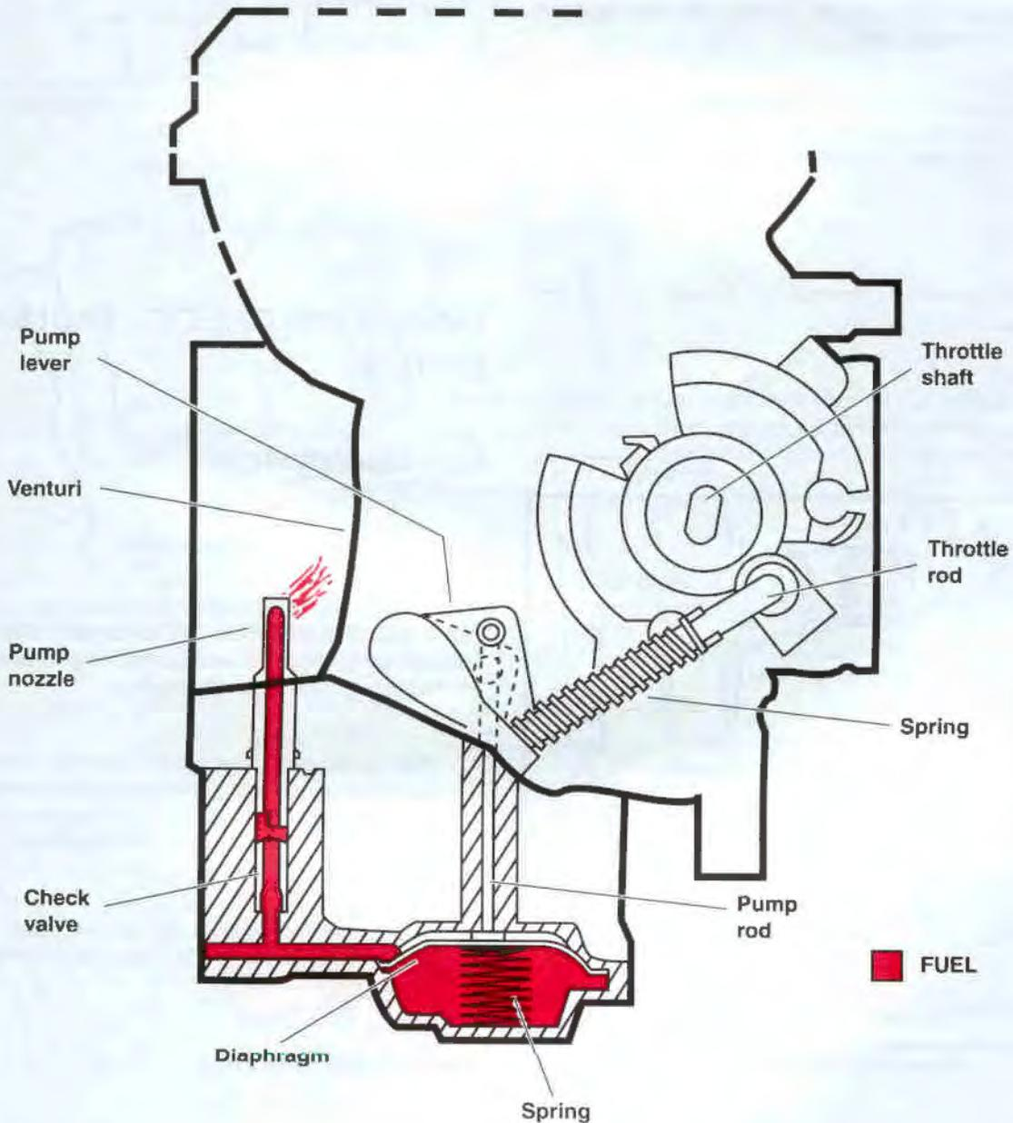
Figure 4-8. Accelerator Pump System
