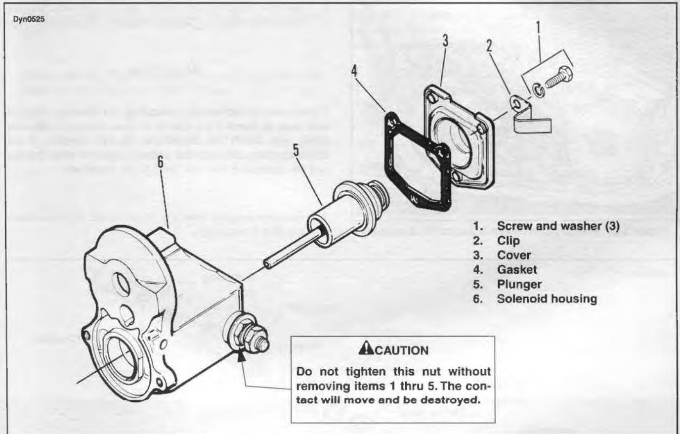
Figure 5-26. Starter Solenoid
