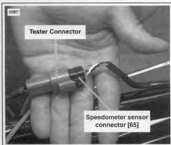
Figure 8-53. Test Connection
