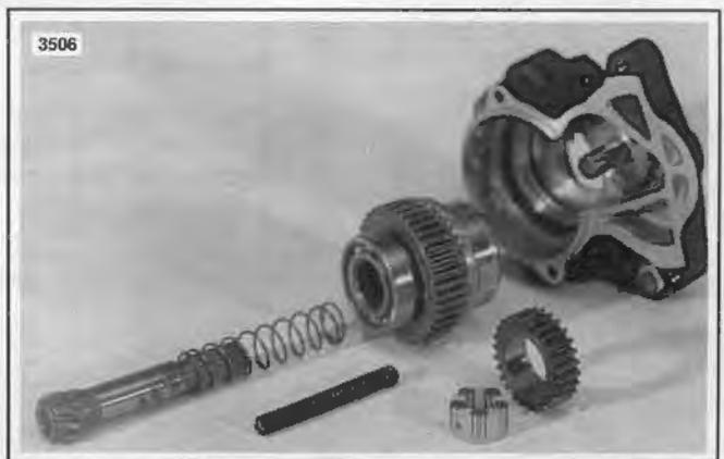
Figure 5-25. Clutch Assembly
