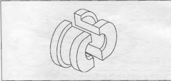
Part No. HD-94547-100 Crankshaft Bearing Outer Race Remover/Installer
