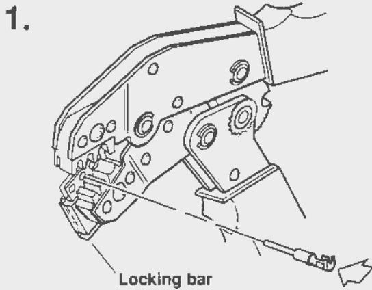
1. Insert contact through middle hole of locking bar.
