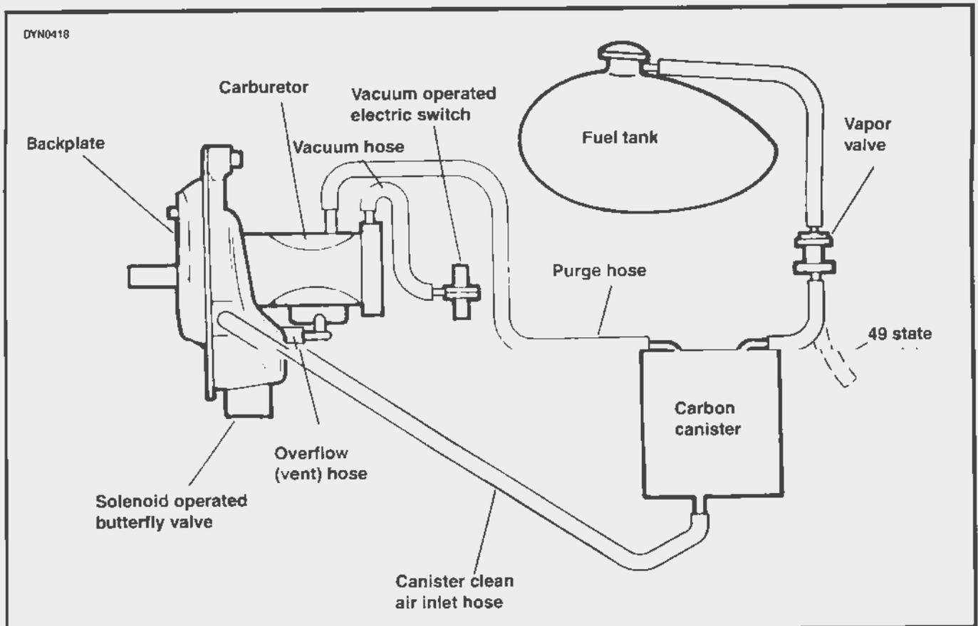
Figure 4-19. Schematic – California Evaporative Emissions Control System
