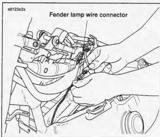
Figure 2-93. Wire Connector– FLSTS
