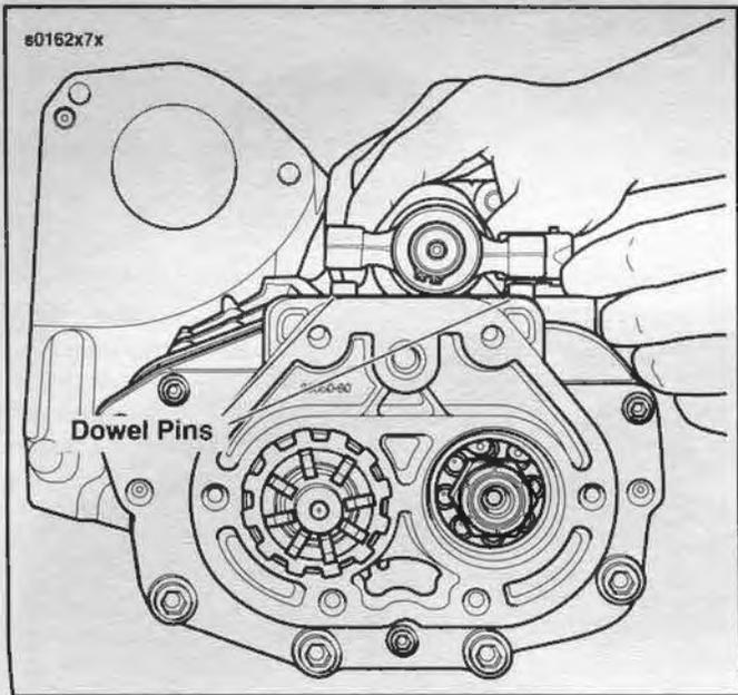
**Figure 7-7. Shifter Cam Support Block Locating Dowel Pins**
