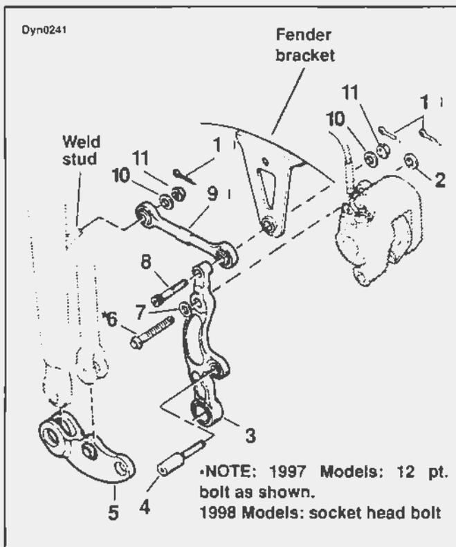
Figure 2-52. Brake Mounting (1997 Model Shown)
