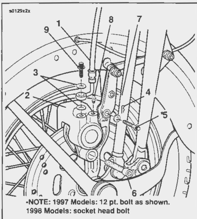
Figure 2-54. Brake Mounting -FLSTS (1997 Model Shown)
