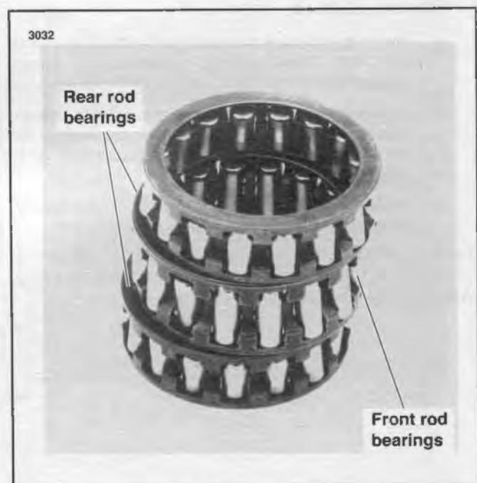
Figure 3-77. Crank Pin Bearing Set
