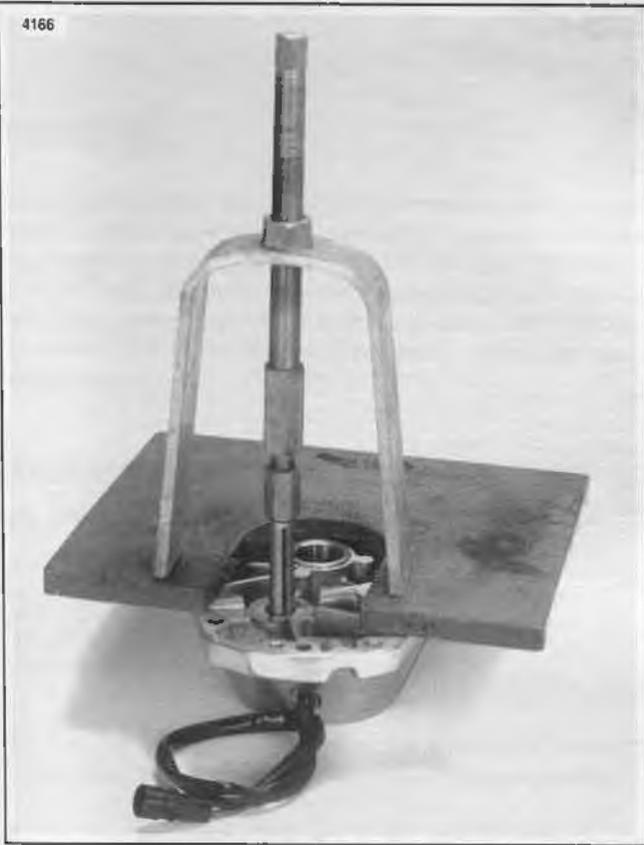
Figure 3-60. Remove Cover Bushing
