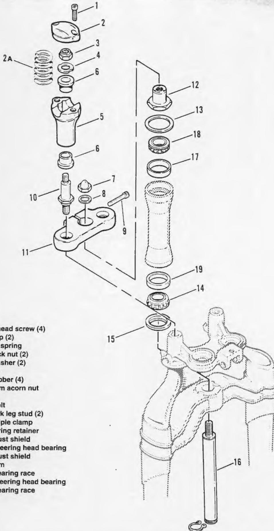
Figure 2-60. Springer Fork (FXSTS, FXSTSB)-1 of 2
