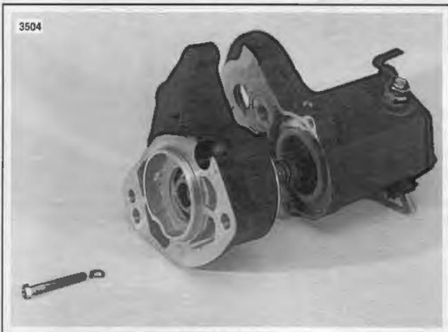
Figure 5-23. Remove Drive Housing
