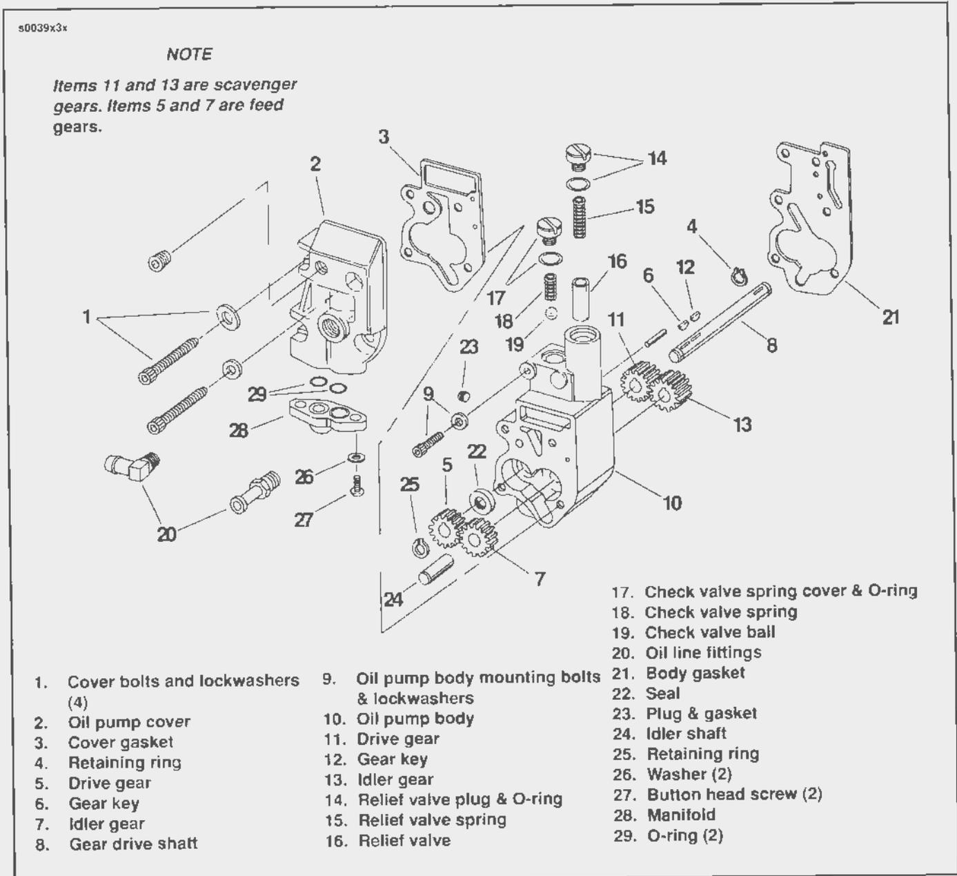
Figure 3-42. Engine Oil Pump
