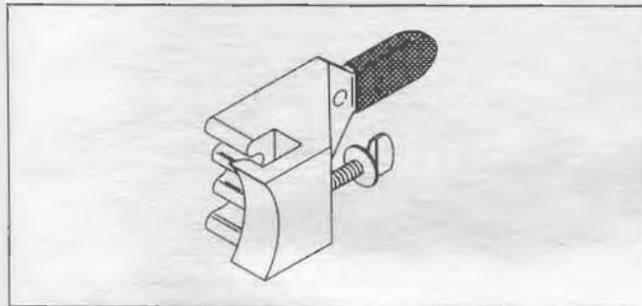
Part No. HD-41184 Sprocket Holding Tool
