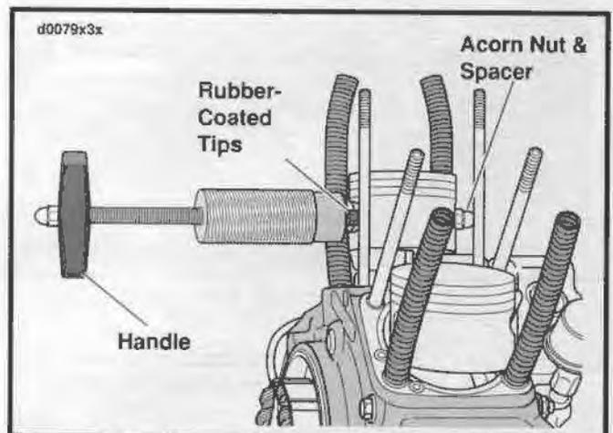
Figure 3-33. Piston Pin Remover/Installer Part No. HD-42320
