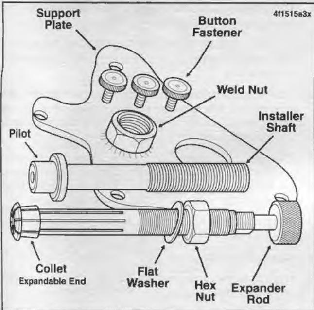
Figure 3-57. Cam Needle Bearing Remover/Installer (Part No. HD-42928)
