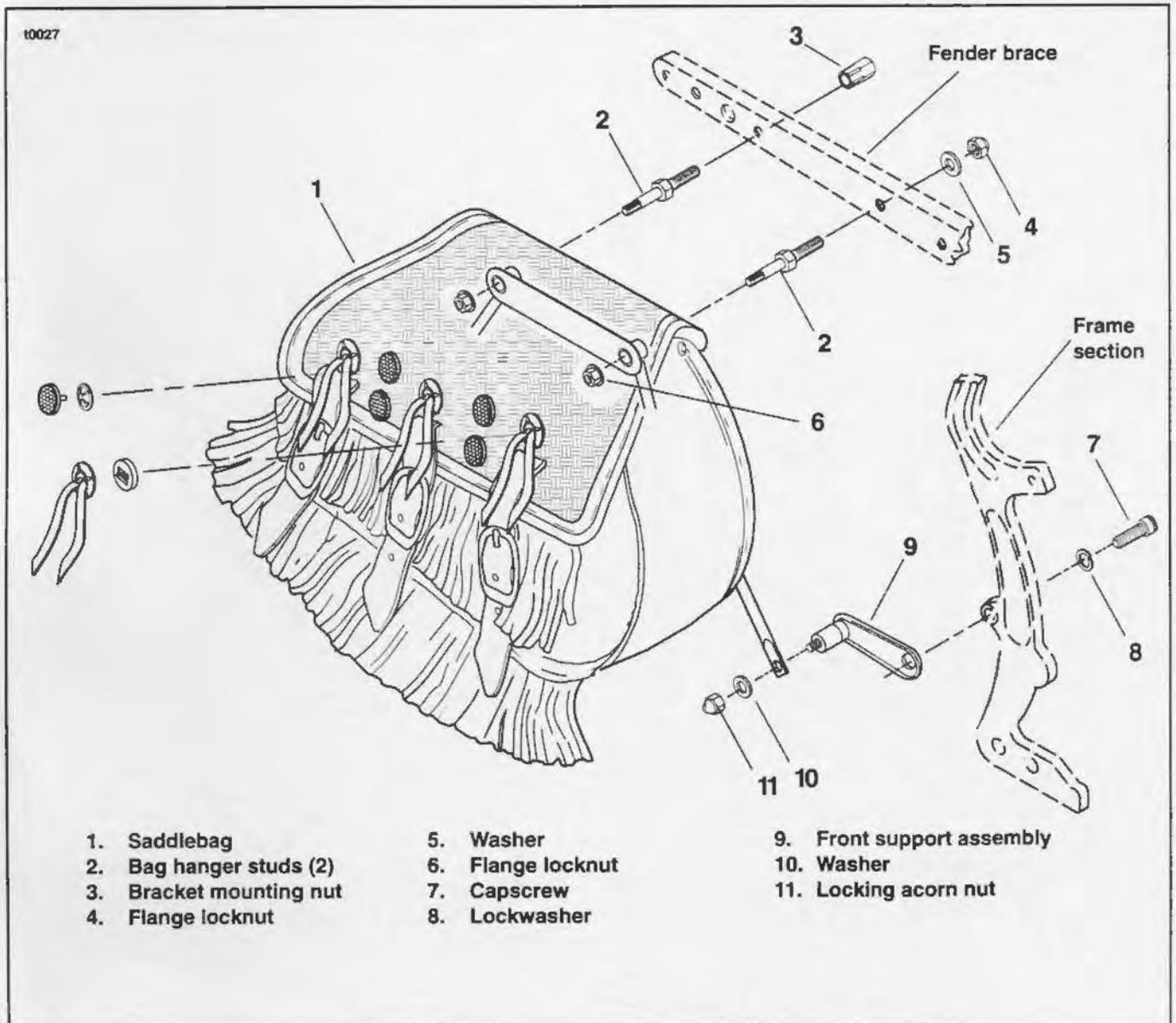
Figure 2-105. Saddlebags and Saddlebag Brackets - FLSTS
