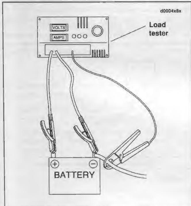
Figure 8-16. Check Current Draw (Ignition Switch on)
