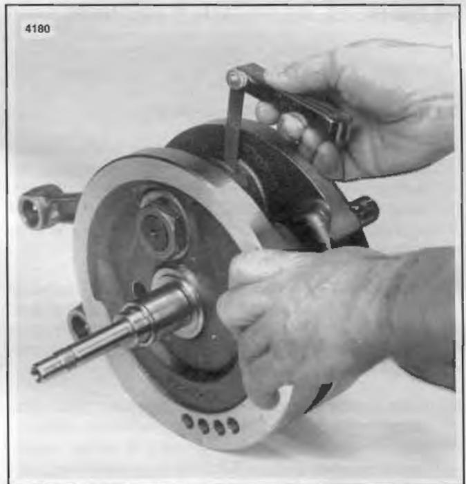
**Figure 3-75. Checking Connecting Rod Side Play**
