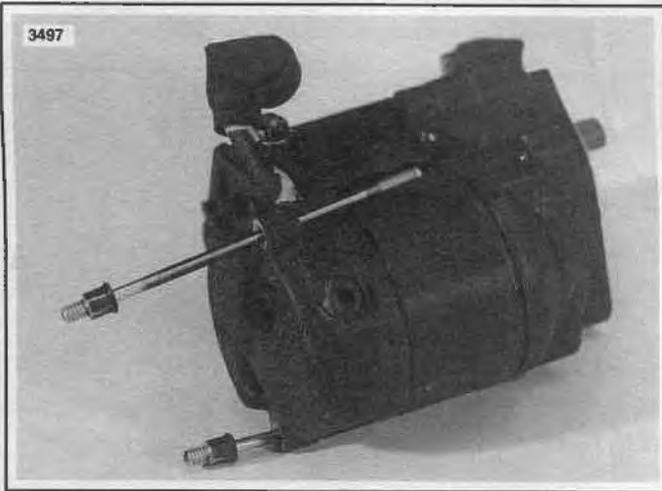
Figure 5-11. Remove Thru-Bolts
