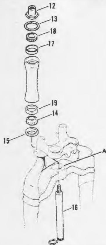
Figure 2-81. FXSTS, FXSTSB, FLSTS Steering Head Assembly
