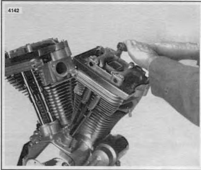
**Figure 3-10. Remove Lower Rocker Arm Cover Fasteners**
