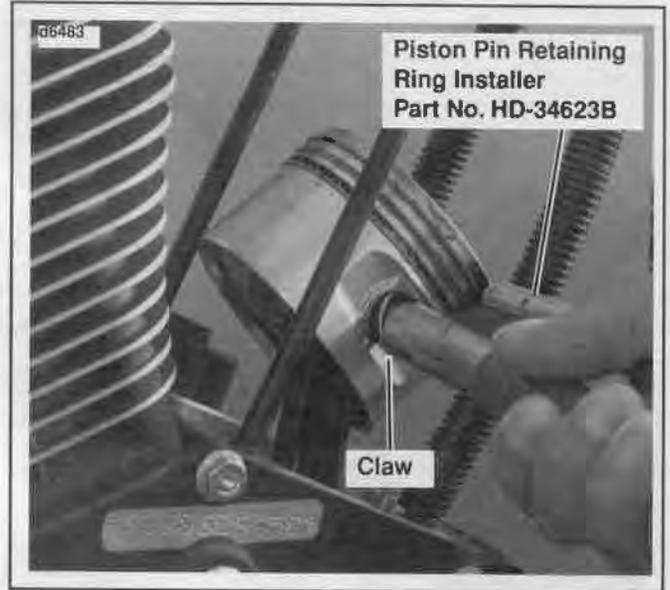
Figure 3-32. Remove /Install Piston Pin Retaining Ring
