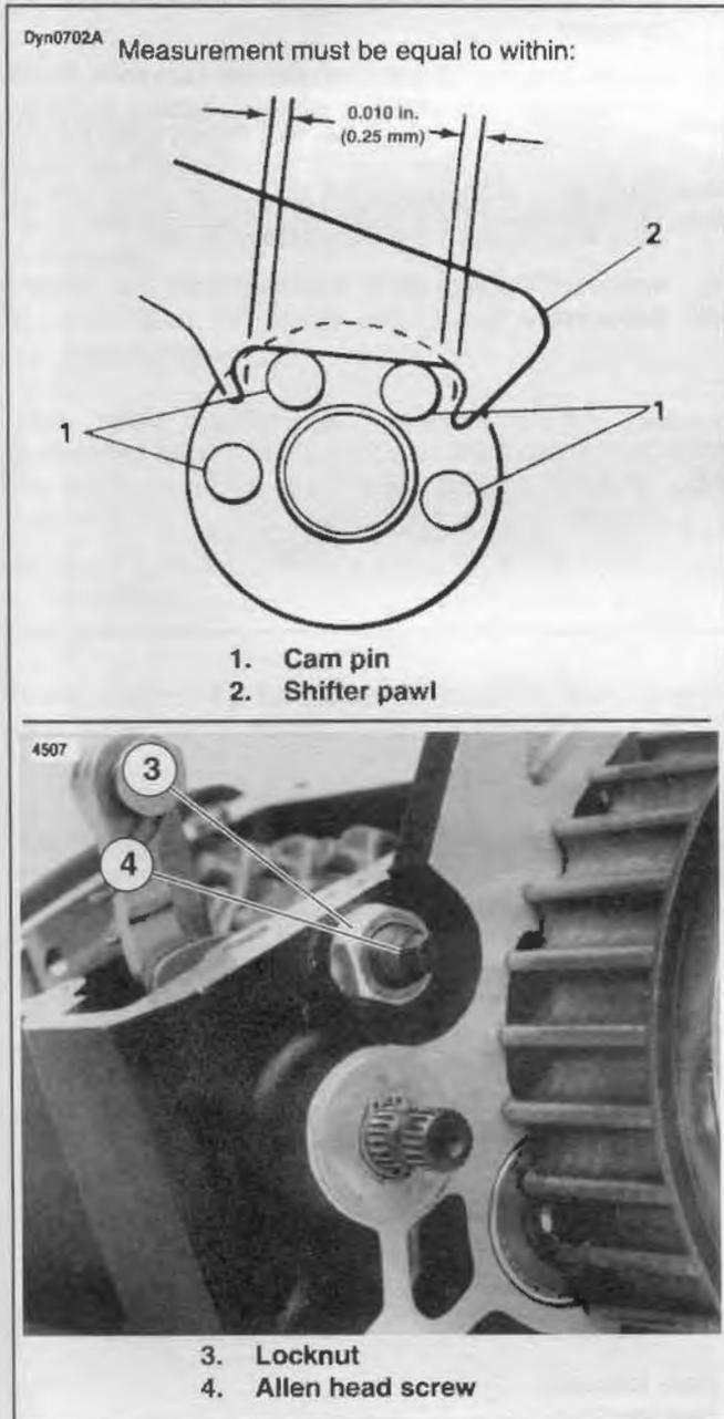
Figure 7-3. Gear Engagement Adjustment
