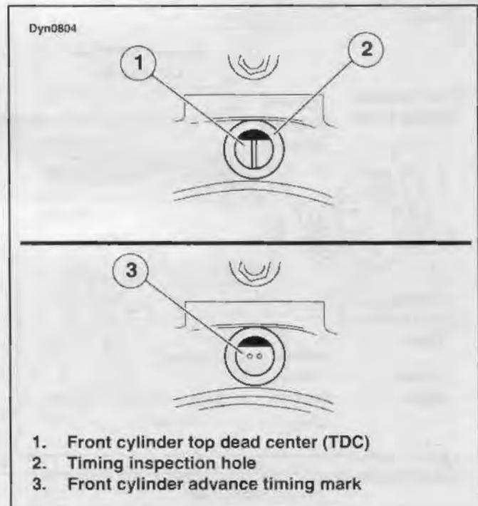
Figure 8-4. Ignition Timing Mark
