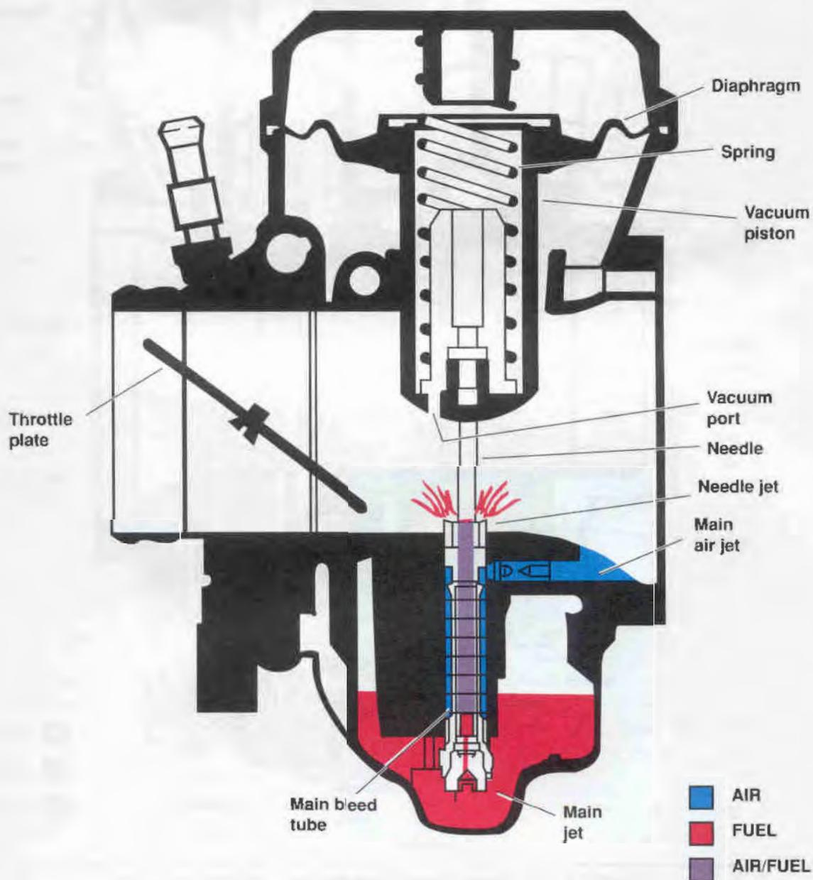
Figure 4-6. Mid Range Slide Position and Fuel Discharge
