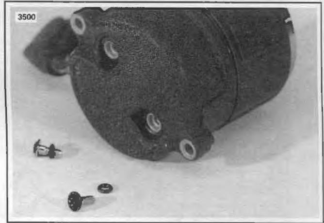
Figure 5-13. Remove End Cap Screws & O-rings
