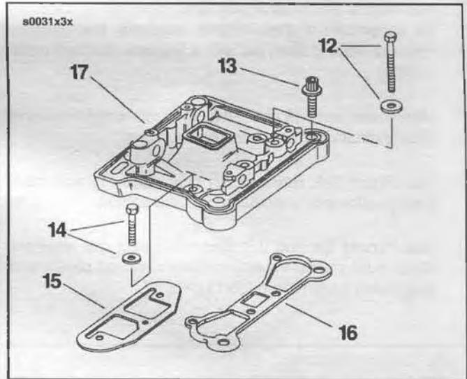
**Figure 3-11. Lower Rocker Arm Cover and Gasket**
