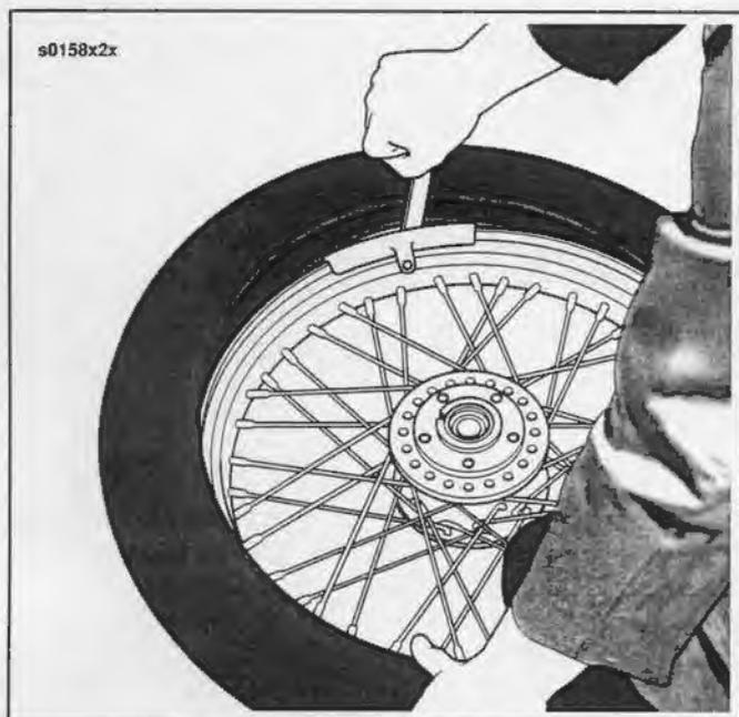
Figure 2-37. Starting Bead on Rim
