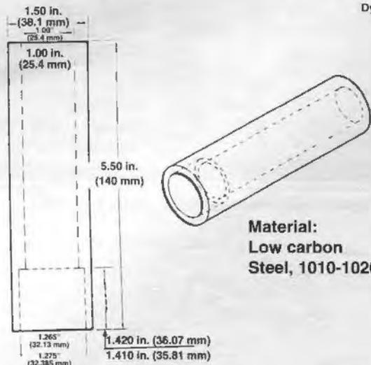
Figure 3-84. Inner Race Installation Tool
