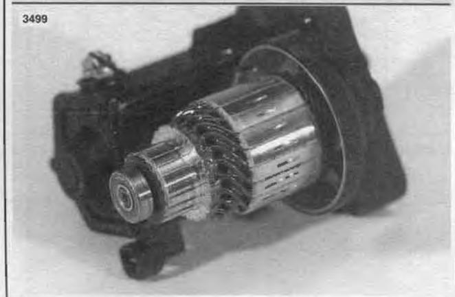
Figure 5-12. Remove Field Coil and Cap
