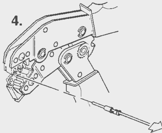
4. Raise locking bar and remove contact.
