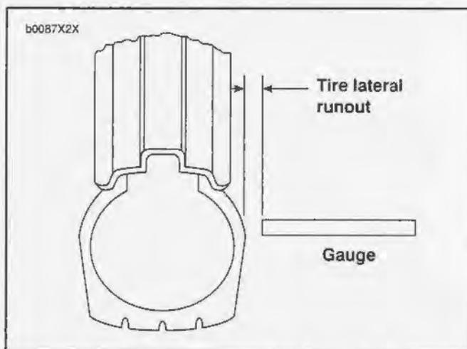
Figure 2-39. Checking Tire Lateral Runout
