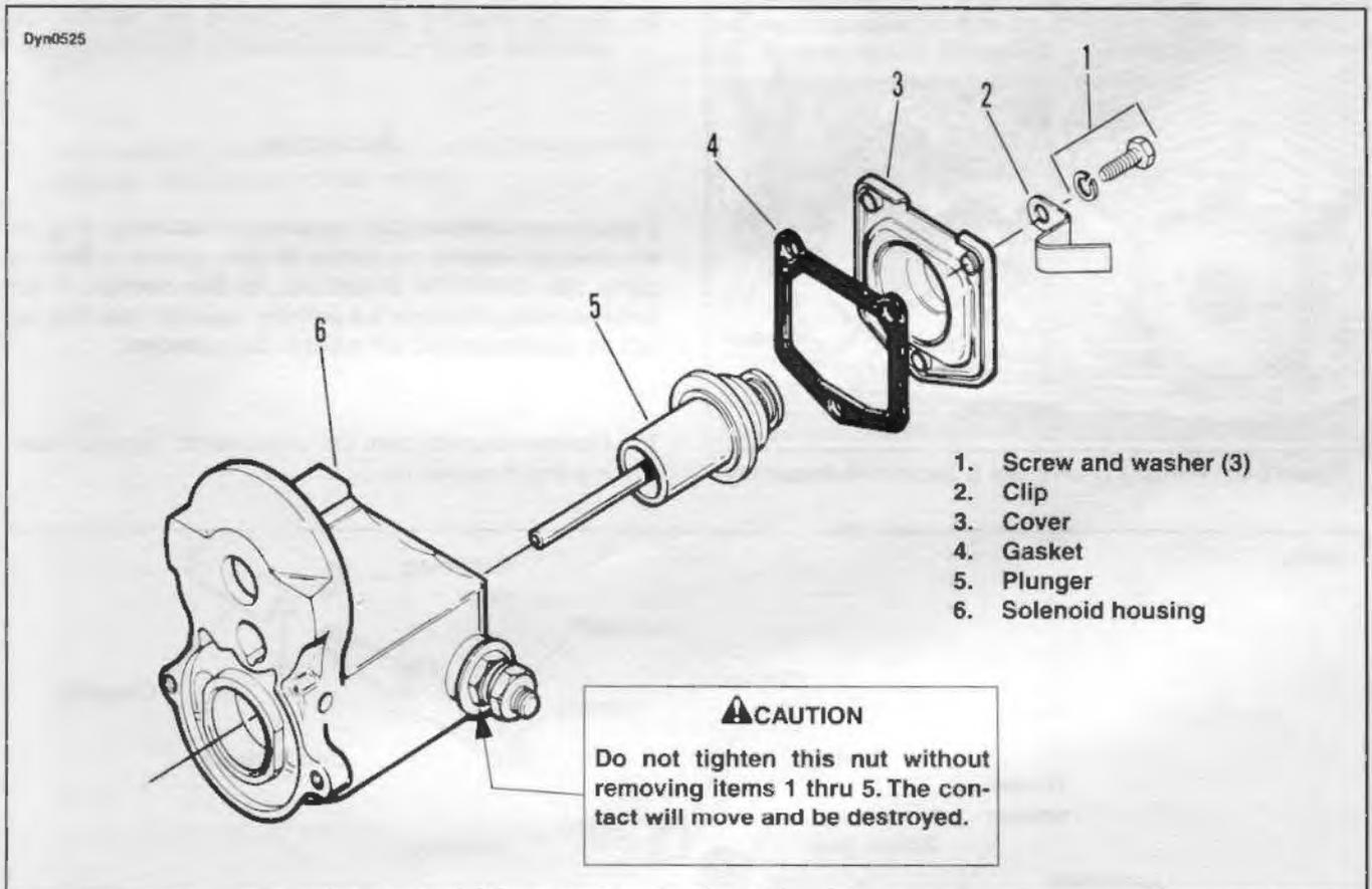
Figure 5-26. Starter Solenoid
