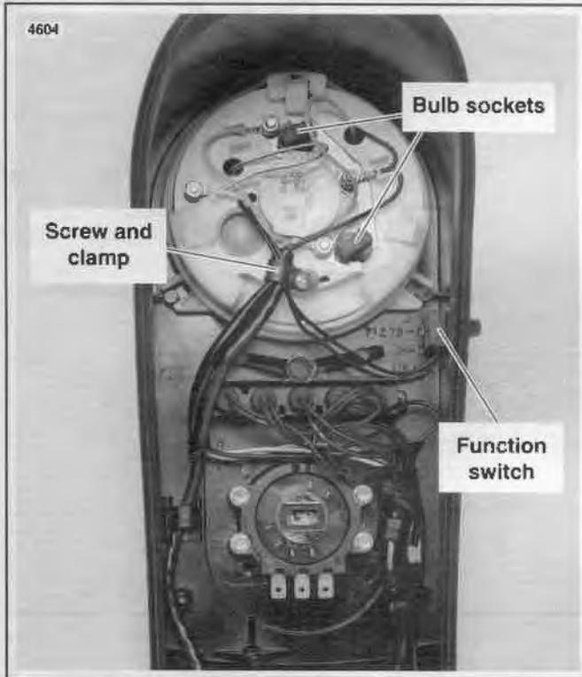
Figure 8-49. Electronic Speedometer
