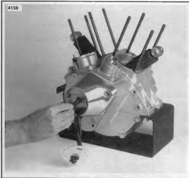
Figure 3-52. Remove Gear Cover
