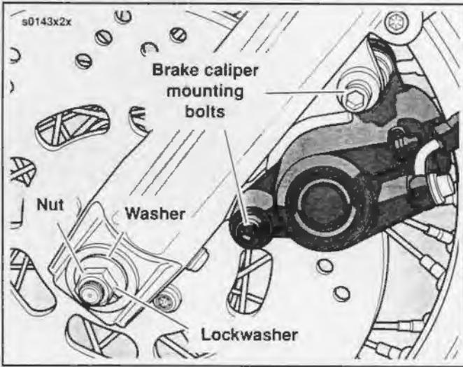
Figure 2-1. Front Wheel Mounting (left side FXSTC shown)
