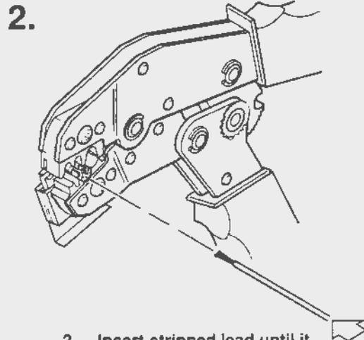
2. Insert stripped lead until it contacts locking bar.
