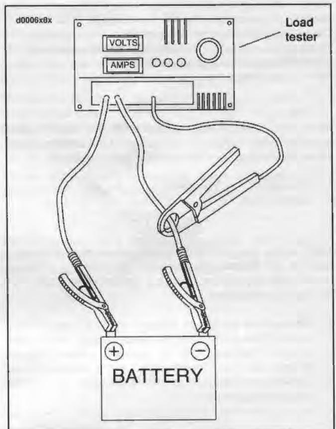
Figure 8-25. Load Test
