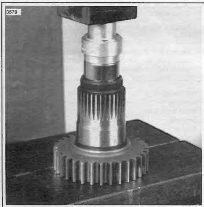
**Figure 7-28. Installing Clutch Side Needle Bearing in Main Drive Gear**
