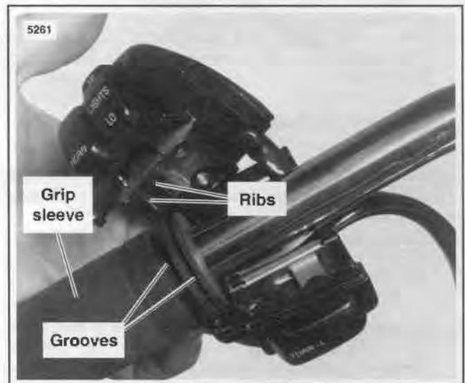
Figure 8-66. Install Left Handlebar Switch Housings
