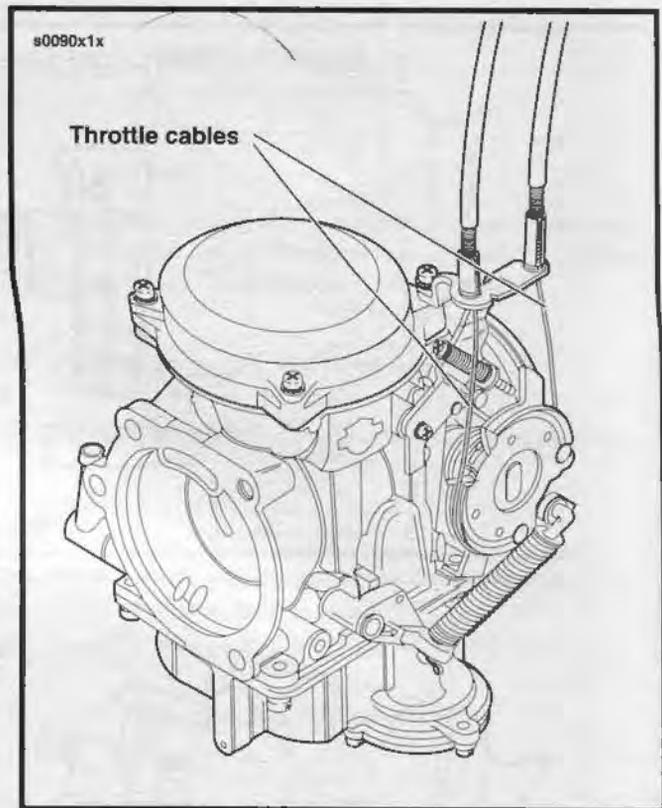
Figure 4-11. Throttle Cables
