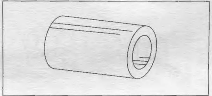
Part No. HD-34731 Shoulderless Valve Guide Installer
