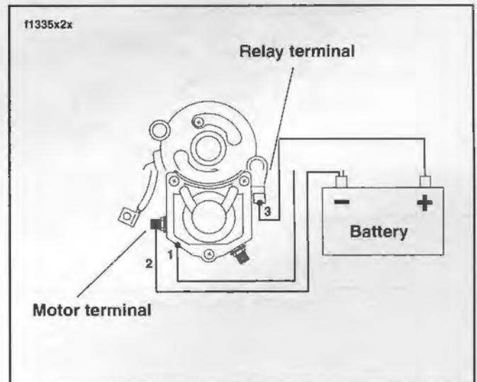
Figure 5-6. Pull-In Test
