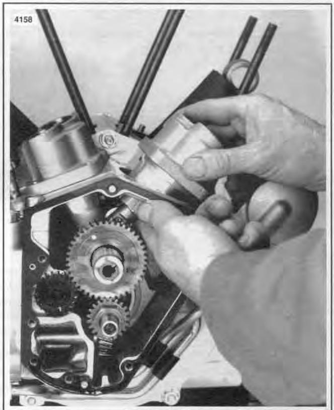
Figure 3-49. Lifter Assembly
