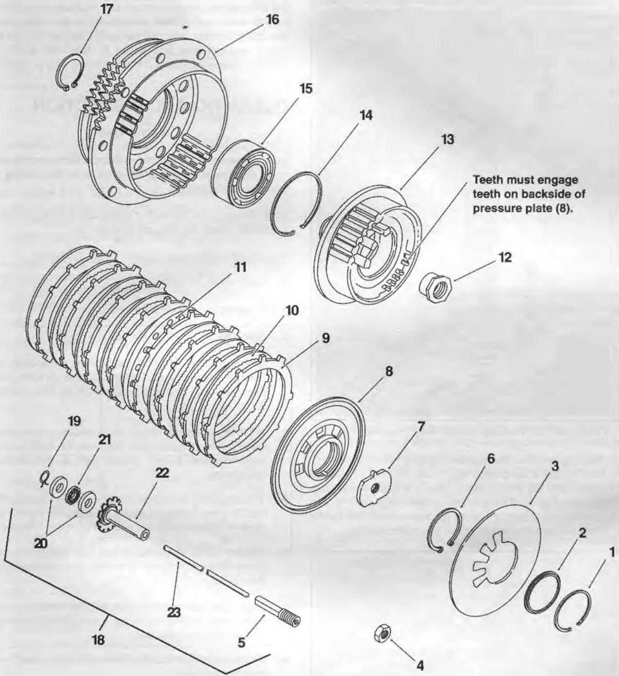
Teeth must engage teeth on backside of pressure plate (8).
