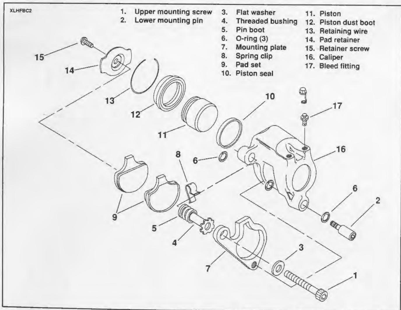
Figure 2-49. Front Brake Caliper
