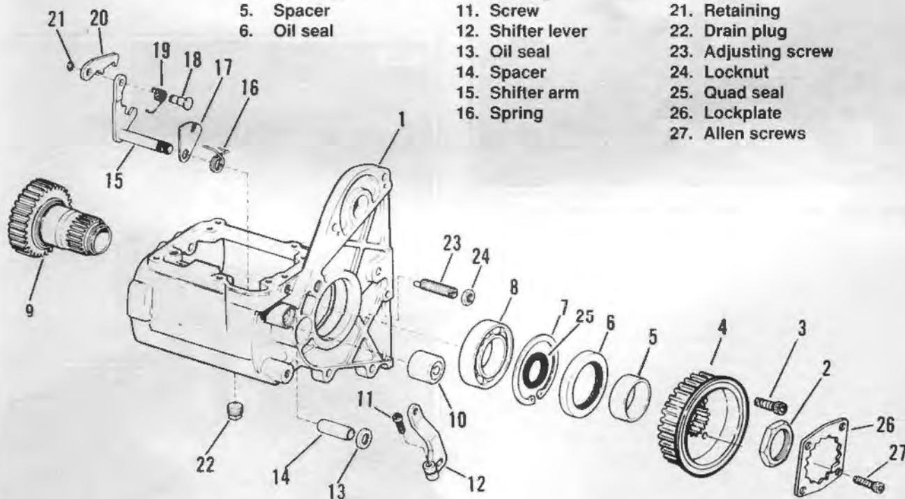
Figure 7-27. Transmission Case, Sprocket and Main Drive Gear
