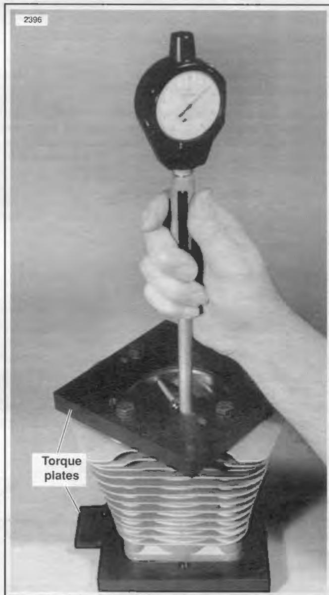
Figure 3-36. Measure Cylinder Bore
