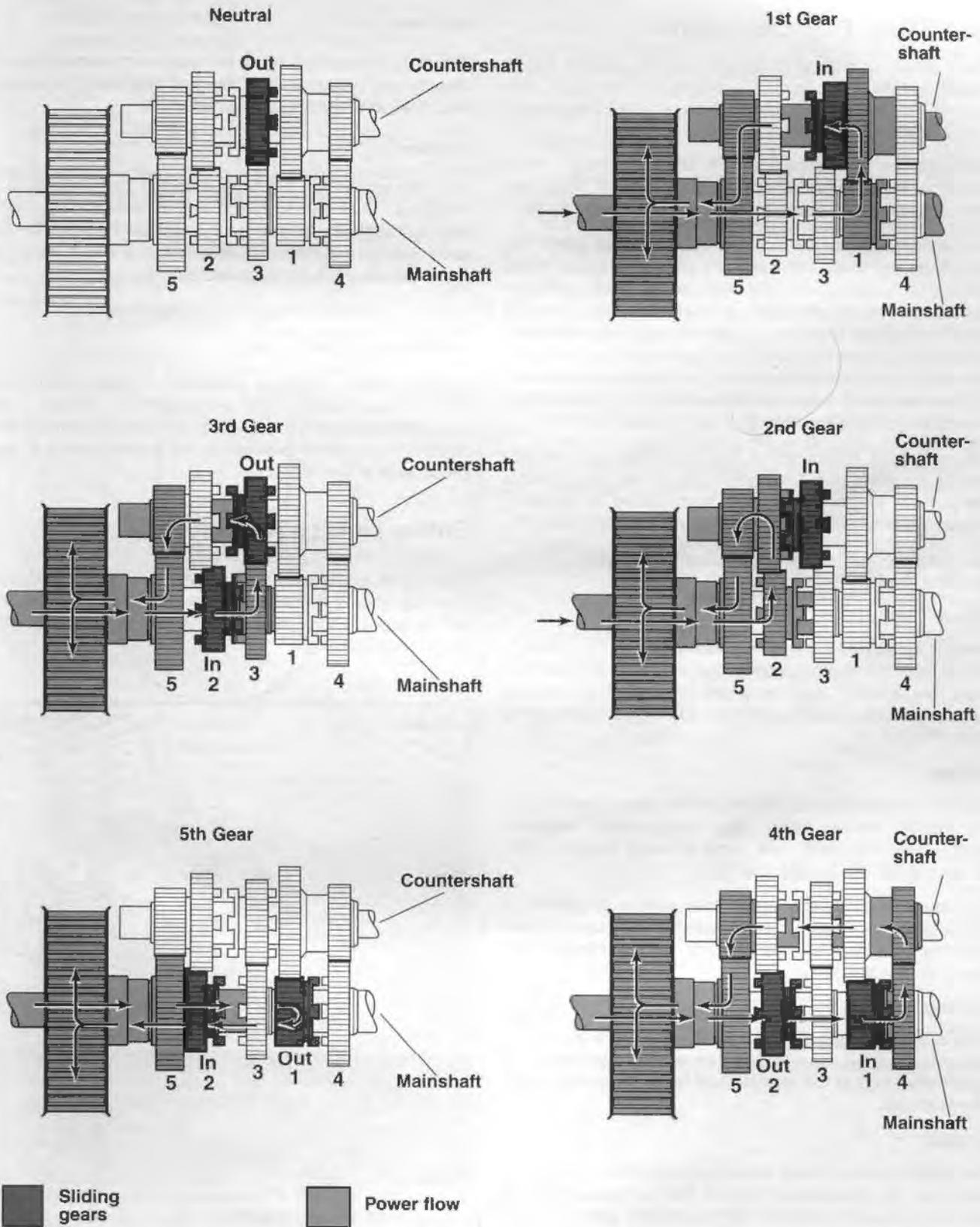
Figure 7-1. Transmission Power Flow
