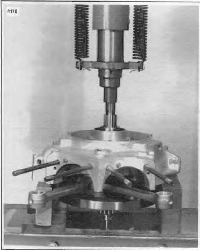
Figure 3-66. Pressing Flywheels Out of Crankcase
