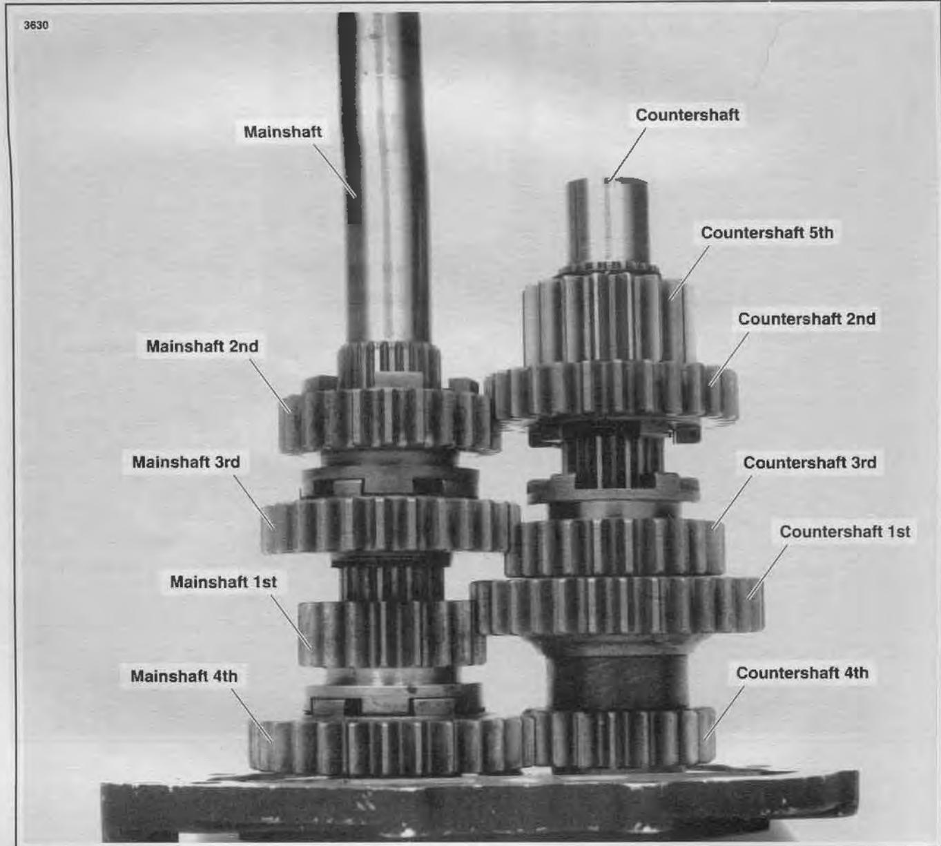
**Figure 7-24. Side Door, Mainshaft and Countershaft – Final Assembly**
