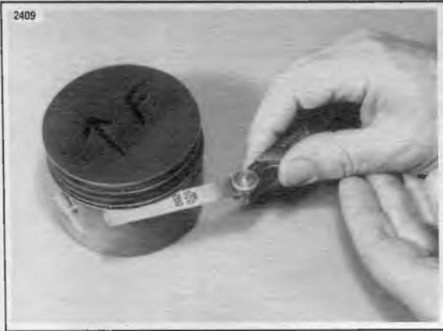
Figure 3-39. Measure Ring Side Clearance
