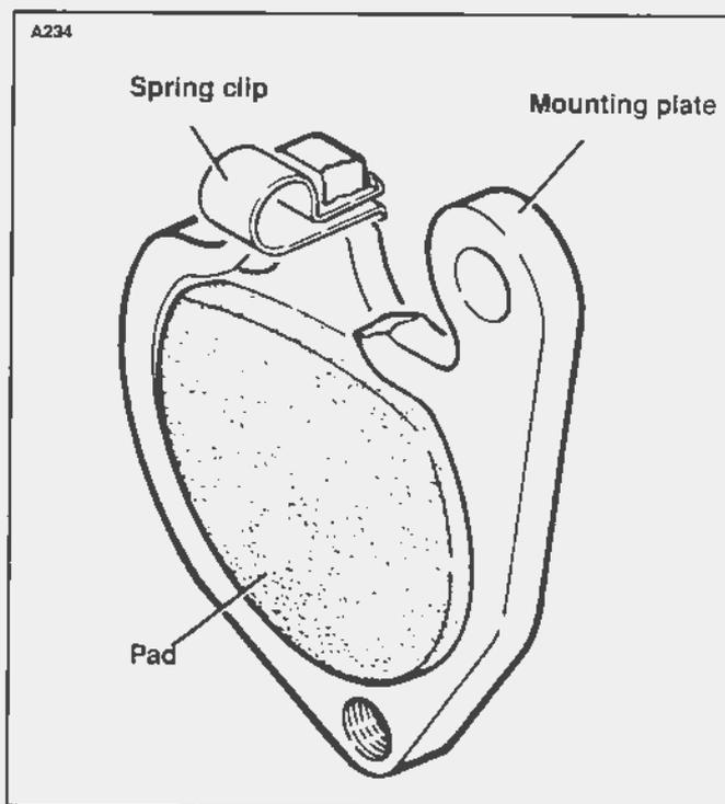
**Figure 2-51. Spring Clip Installation**
