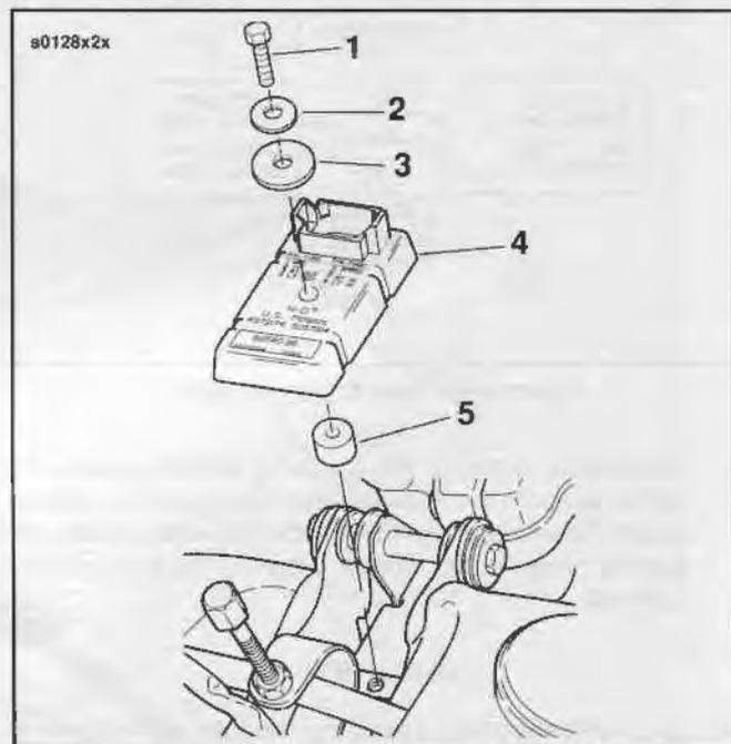
Figure 8-44. Softtail Turn Signal Module
