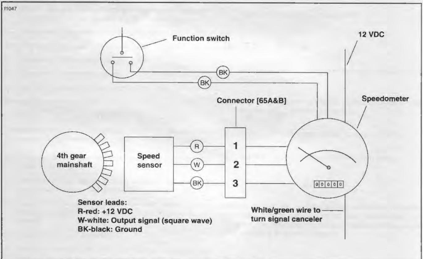
Figure 8-47. Electronic Speedometer Connectors
