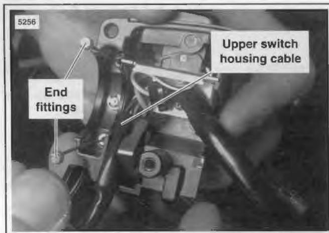
**Figure 8-62. Route Cable to Upper Switch Housing**
