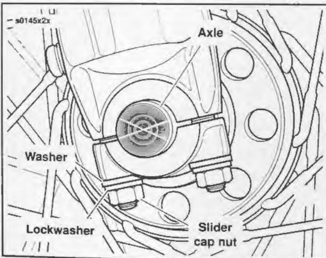
Figure 2-2. Front Wheel Mounting (FLSTC right side)
