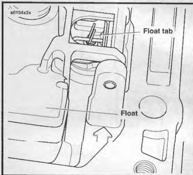
Figure 4-9. Carburetor Float
