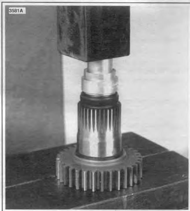
**Figure 7-29. Press in Seal**
