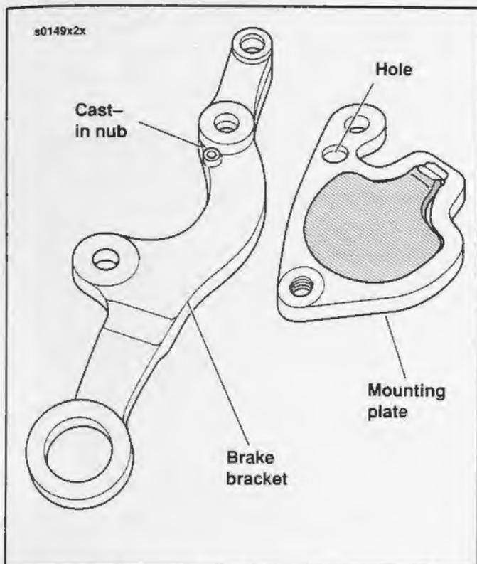
Figure 2-53. Springer Brake Bracket and Mounting Plate
