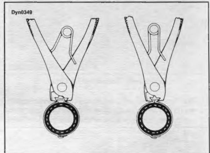
Figure 3-45. Hose Clamps and Hose Clamp Tool
