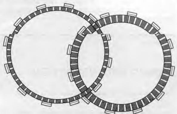
Figure 6-20. Friction Plates
