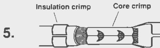
5. Inspect quality of core and insulation crimps.
