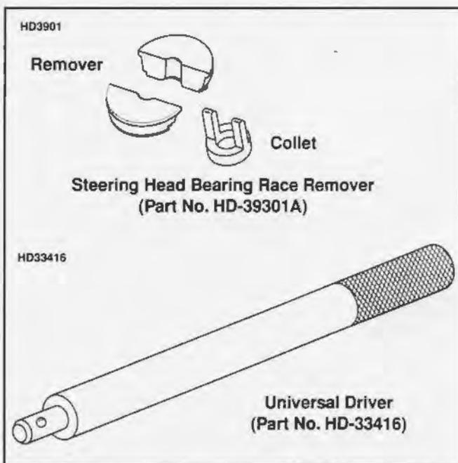
Figure 2-82. Steering Head Bearing Race Removal Tools
