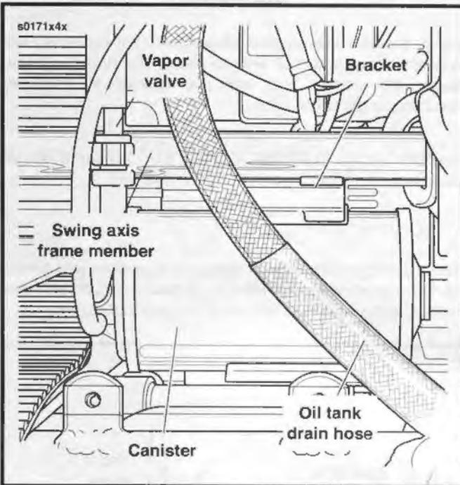
Figure 4-20. EVAP Canister (rear wheel removed for clarity)
