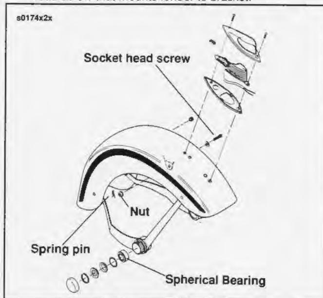
Figure 2-94. Front Fender – FLSTS
