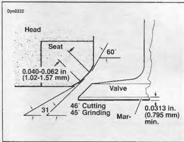
Figure 3-28. Valve Seat Angles
