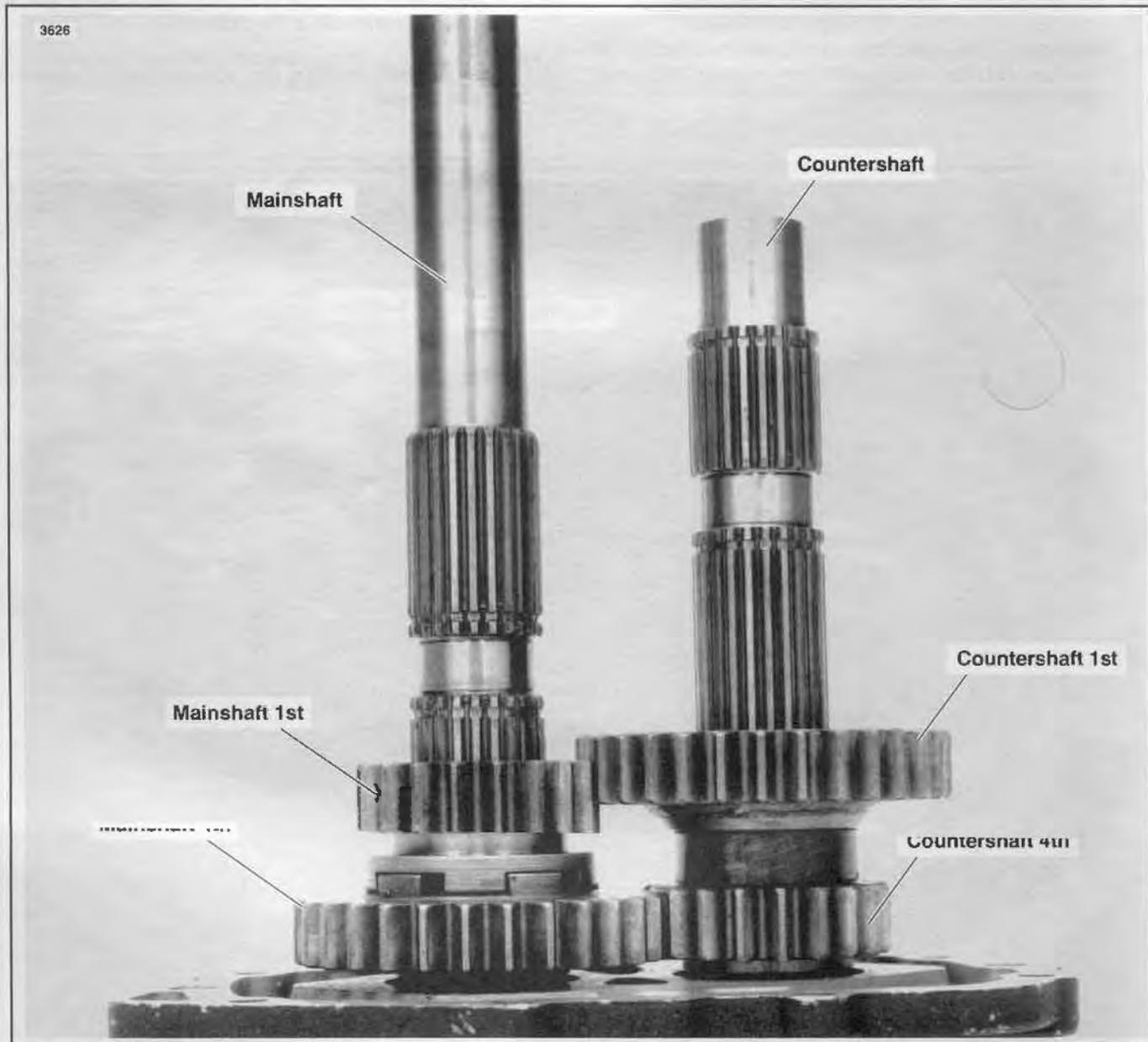
Figure 7-20. 4th and 1st Gears on Shafts
