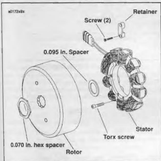
Figure 8-22. Rotor and Stator Mounting
