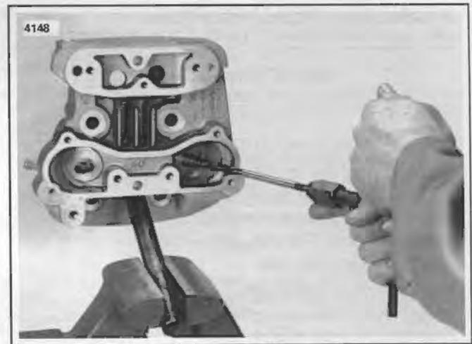
Figure 3-26. Ream Valve Guide
