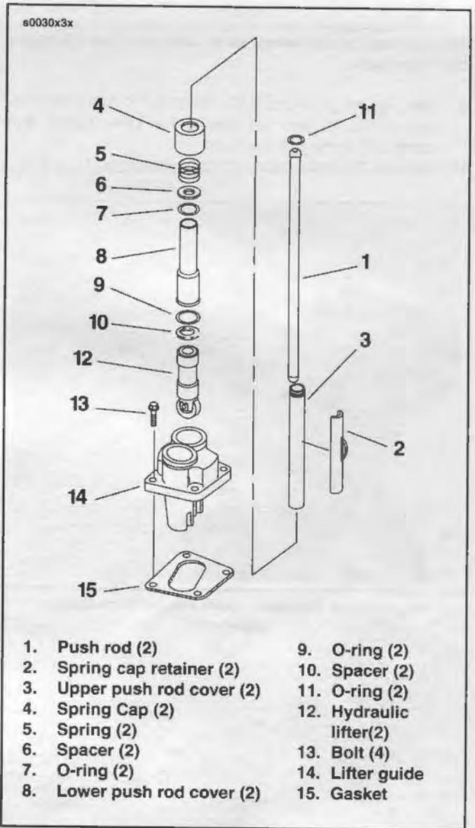
Figure 3-9. Rocker Arm Push Rod and Cover
