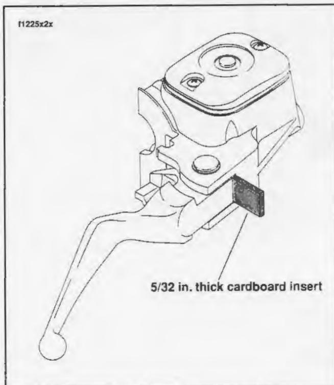
Figure 2-44. Install Cardboard Insert Before Removing Master Cylinder Assembly
