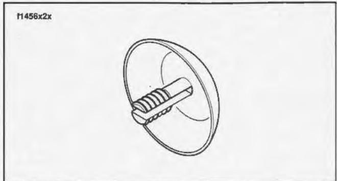
Figure 2-103. Passenger Seat Retention Nut Plug (FLSTS)
