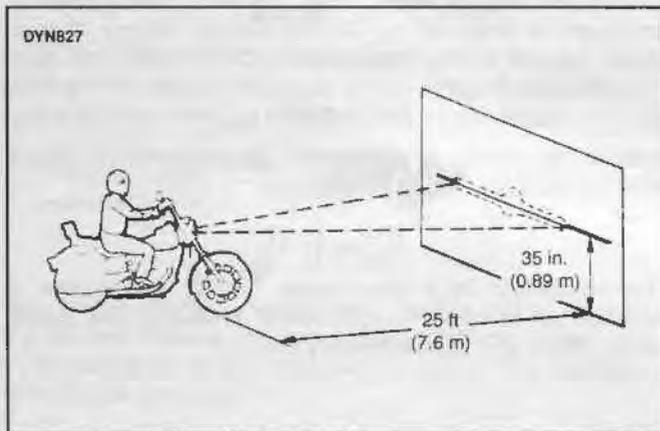
Figure 8-31. Headlamp Adjustment – FXSTC, FXSTS, FXSTSB and FLSTS
