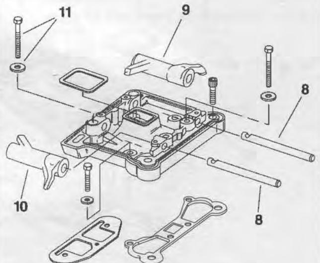
**Figure 3-7. Rocker Arm Retaining Bolts**
