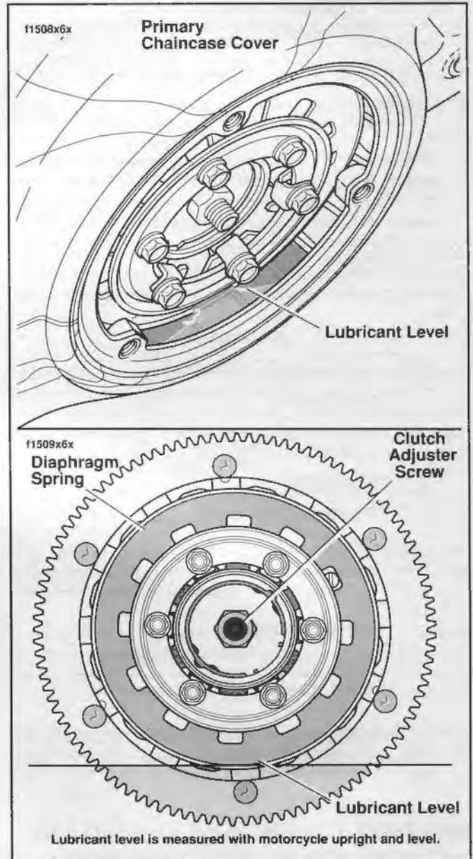
Figure 1-6. 1998 Models Primary Chaincase Lubricant Level
