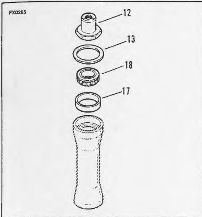
Figure 2-65. Dust Shield and Hex Bearing Retainer
