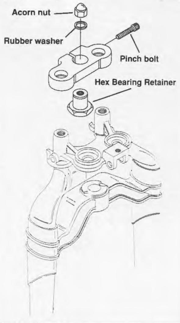
Figure 2-77. Handlebar Risers Assembly
