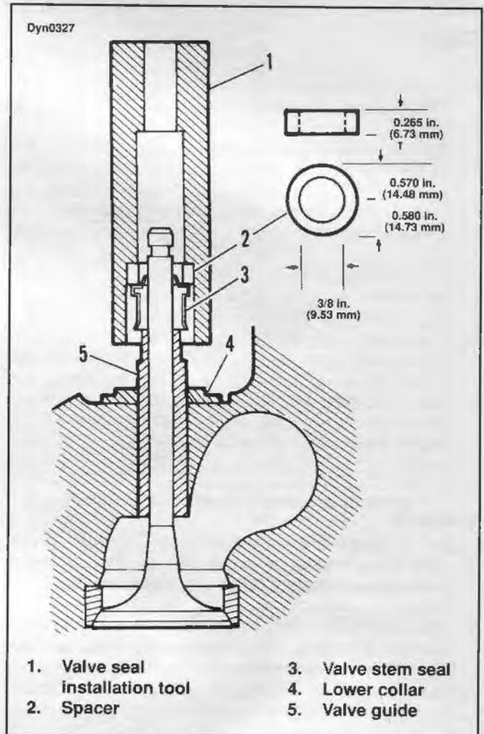
Figure 3-23. Valve Seal Installation With Spacer
