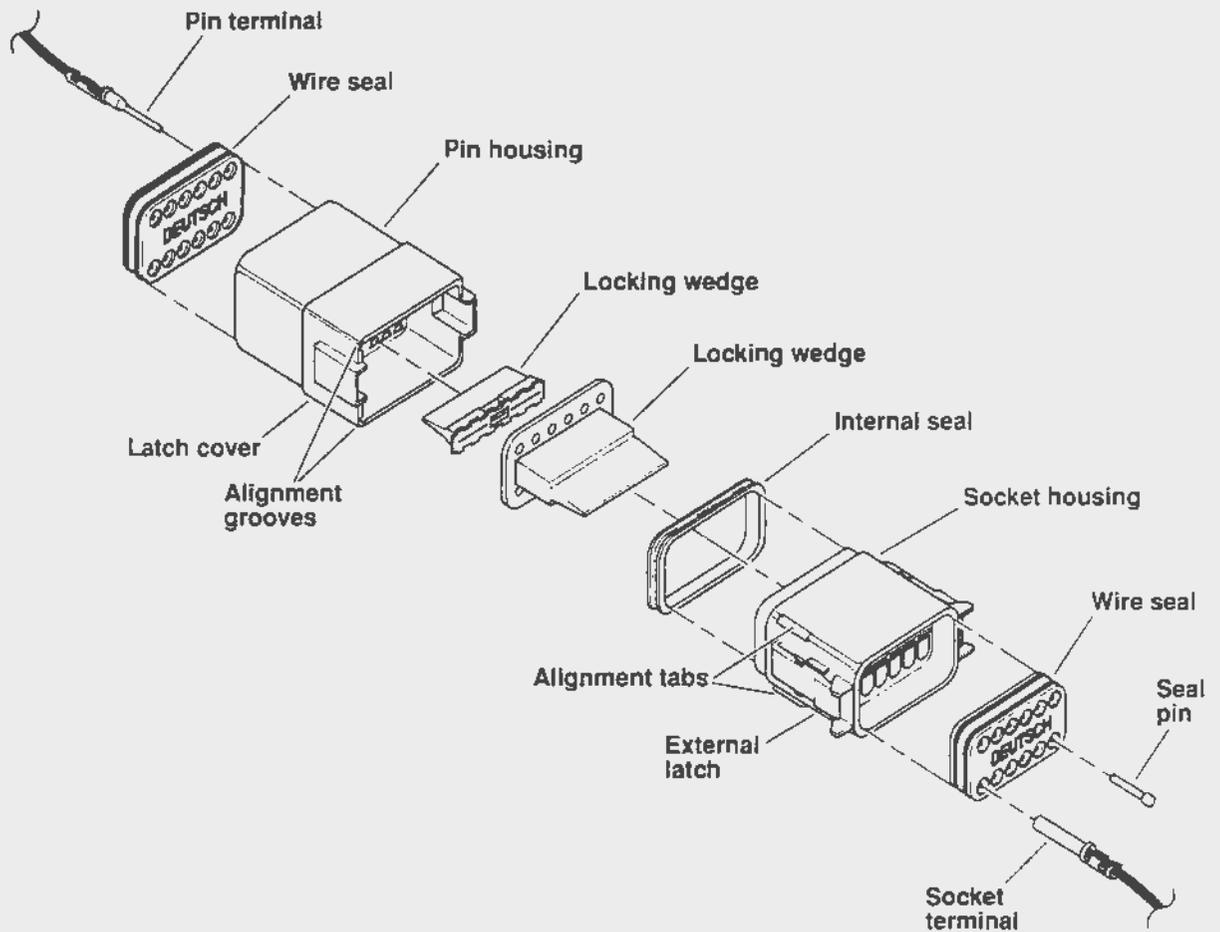
Figure A-8. 12-pin Deutsch Connector (Exploded View)
