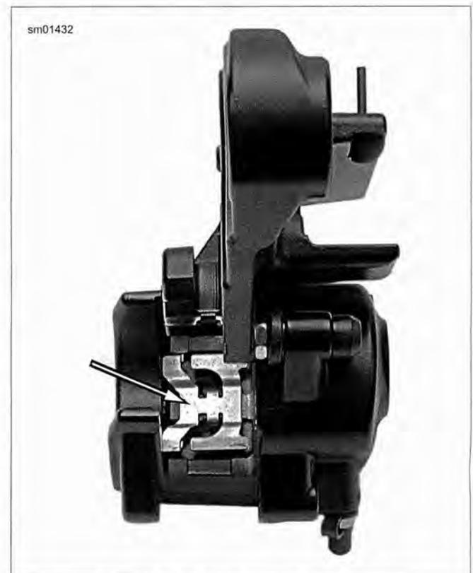
Figure 2-97. Rear Caliper Pad Spring
