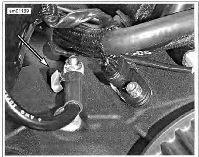
Figure 6-25. Negative Battery Cable Stop on Crankcase (typical)
