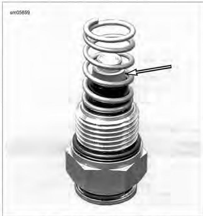
Figure 3-139. Thermostat: XR 1200X
