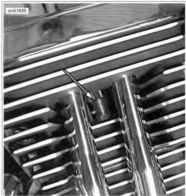
Figure 4-25. Engine Temperature (ET) Sensor Location
