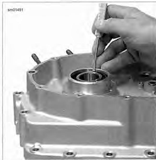
Figure 3-119. Removing Left Main Oil Seal Retaining Ring
