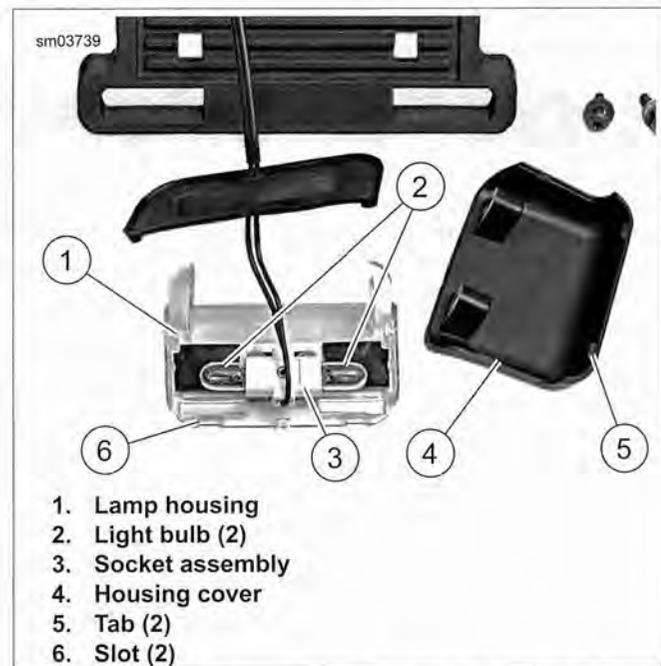
**Figure 6-72. Replacing License Plate Light Bulbs: XL 883N, XL 1200N/X (HDI)**
