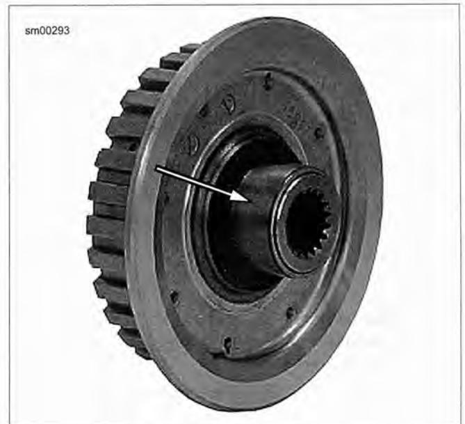
Figure 5-27. Clutch Hub Bearing Race
