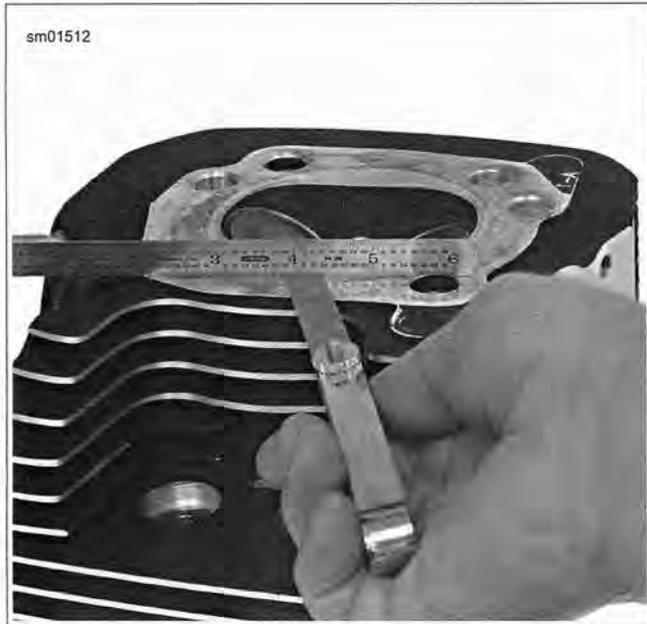
**Figure 3-52. Gasket Surface: Flat Within 0.006 in (0.152 mm)**
