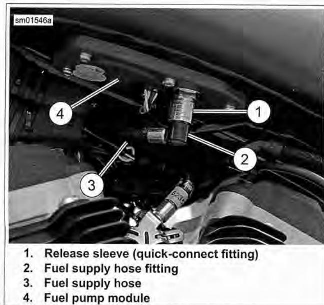
Figure 4-6. Fuel Tank Quick-Connect Fitting
