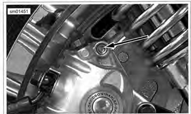
Figure 2-90. Brake Pad Pin (plug removed)
