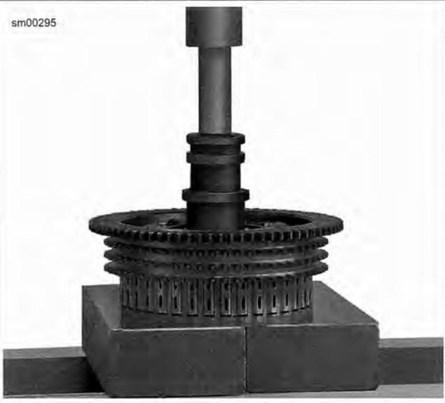
Figure 5-29. Removing Clutch Shell Needle Bearing
