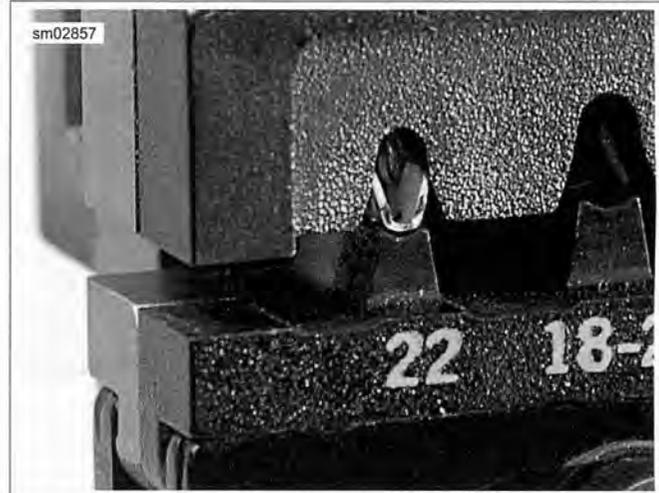
Figure A-52. Crimp Tails in Vertical Alignment between Punch and Die
