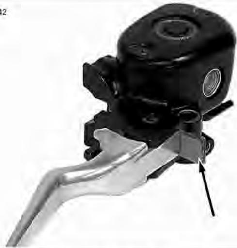
Figure 2-44. Install 5/32 in (4 mm) Cardboard Insert Before Installing Master Cylinder Assembly
