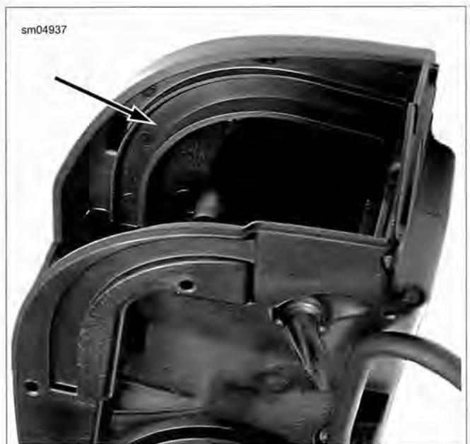
Figure 1-81. Filter Element Channel
