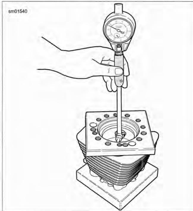
Figure 3-74. Measuring Cylinder Bore
