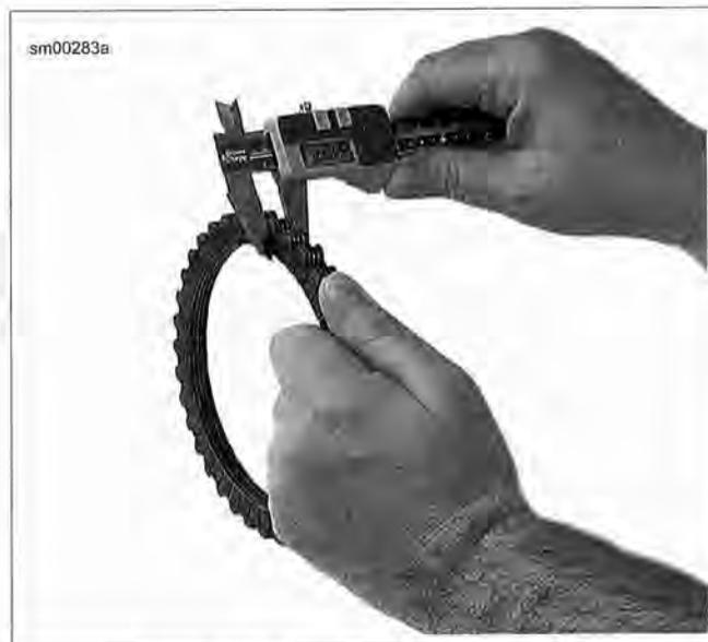
Figure 5-22. Measuring Friction Plates
