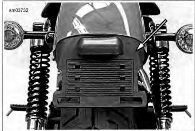
Figure 6-65. License Plate Holder and Lamp Assembly: XL 883N, XL 1200N/X (HDI)
