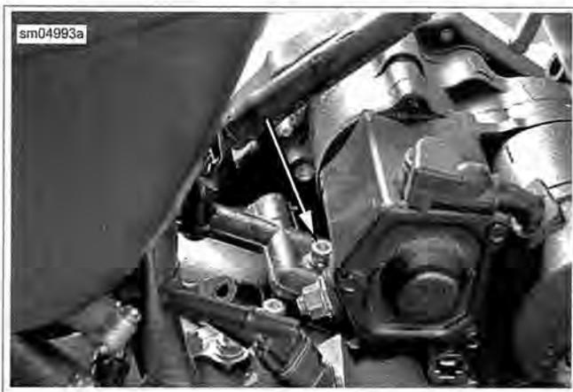
Figure 3-30. Return Oil Manifold Fastener
