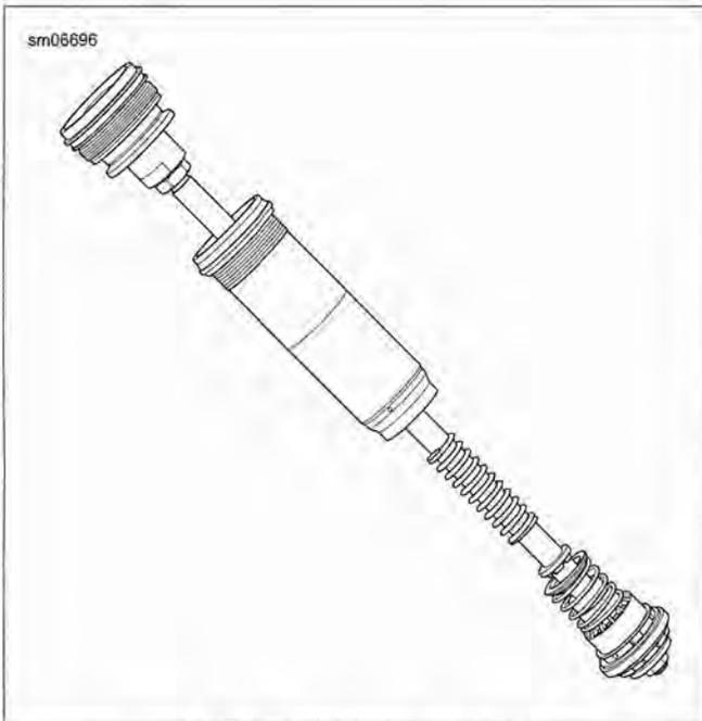
Figure 2-149. Piston Rod Assembly with Rod Case Guide
