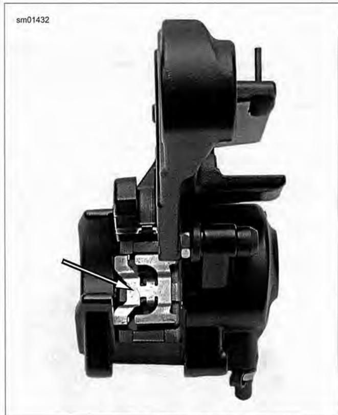
Figure 1-21. Rear Caliper Pad Spring
