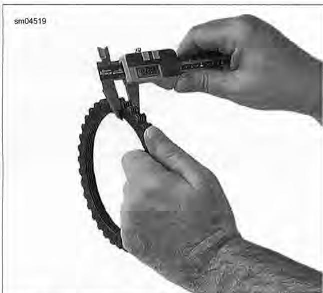
Figure 5-12. Measuring Clutch Friction Plates
