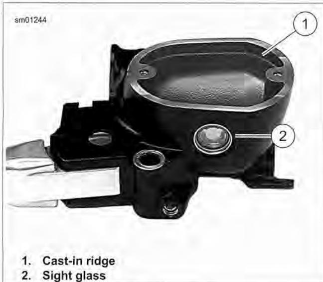
Figure 2-48. Filling Front Master Cylinder Reservoir
