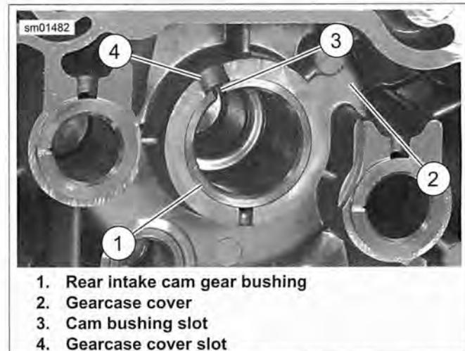
Figure 3-114. Rear Intake Cam Gear Bushing Installed in Gearcase Cover
