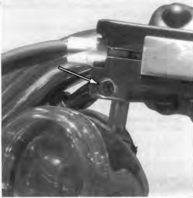
Figure 6-75. Turn Signal Ball Stud Allen Screw
