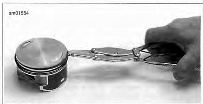
Figure 3-80. Installing Piston Rings (typical)
