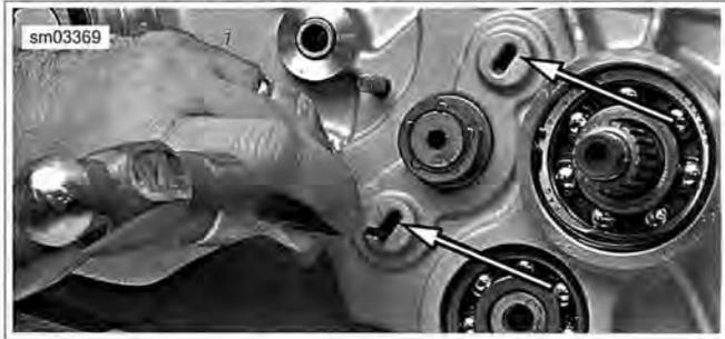
Figure 5-56. Slots For Removing Shifter Fork Shafts
