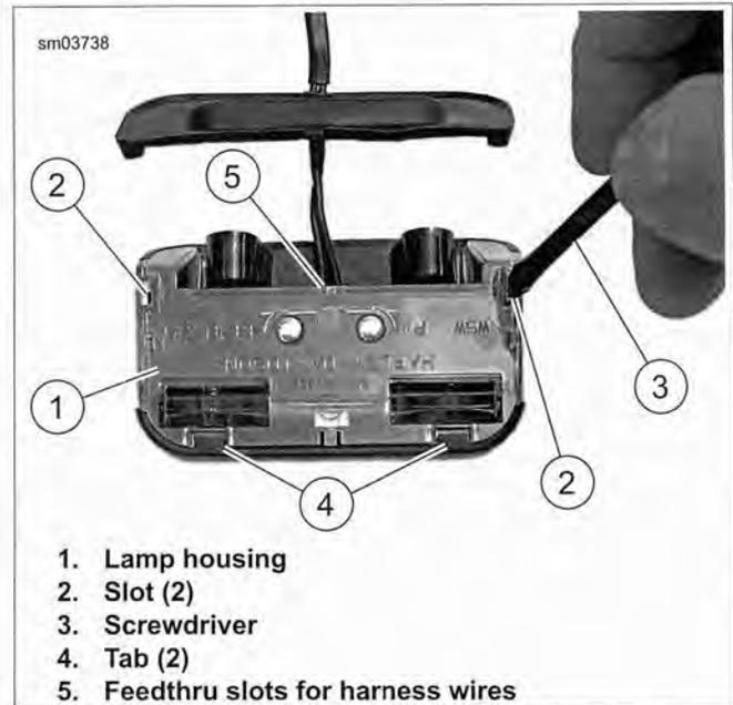
**Figure 6-71. Removing License Plate Lamp Housing Cover: XL 883N, XL 1200N/X (HDI)**
