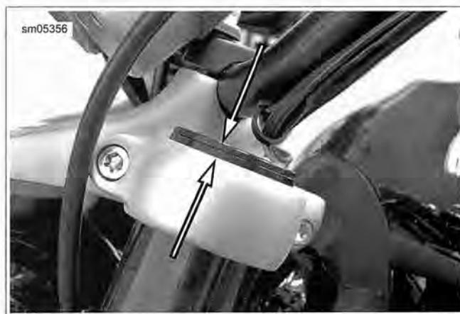
**Figure 2-158. Fork Installation Height Measurement**
