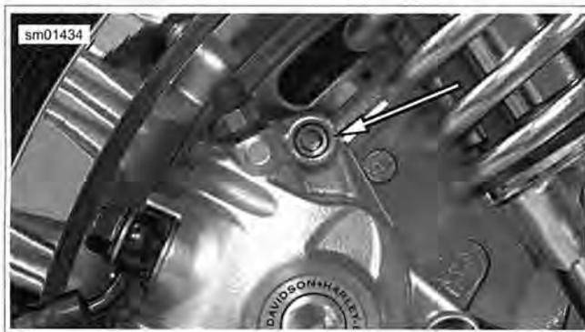
Figure 1-23. Brake Pad Pin (plug removed)
