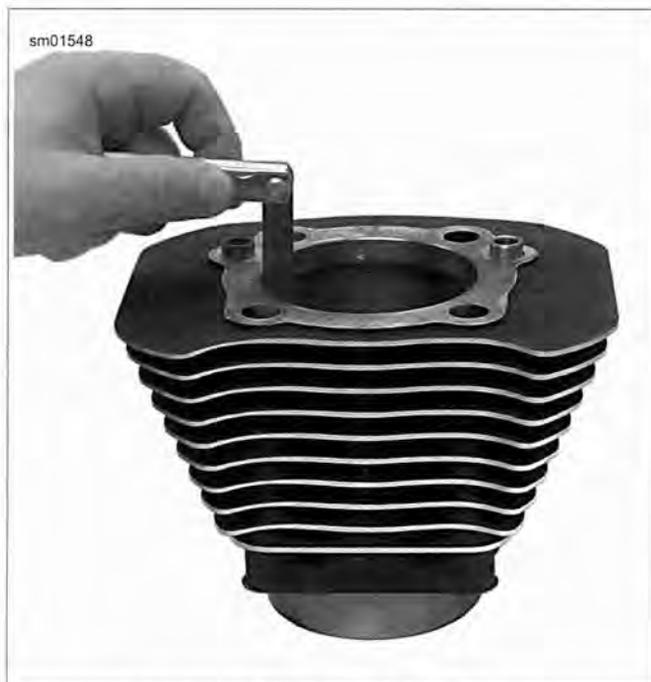
Figure 3-78. Measuring Ring End Gap
