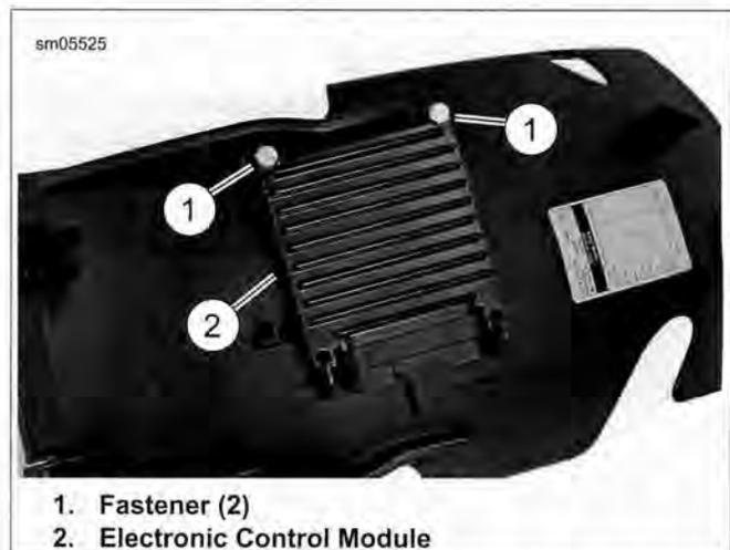
Figure 6-19. Electronic Control Module (ECM): XR 1200X
