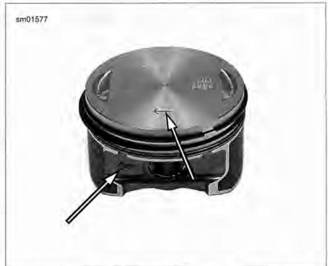
**Figure 3-88. Arrows on Piston Must Point Toward Front of Engine (typical; XL shown)**
