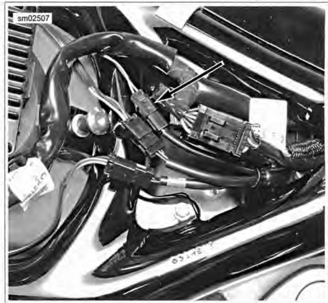
Figure 6-62. License Plate Lamp Connector [40]
