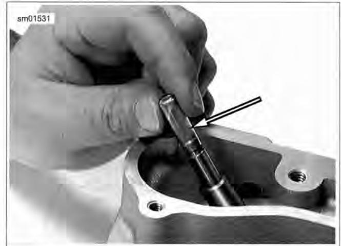
Figure 3-68. Valve Guide Seal Protector Sleeve
