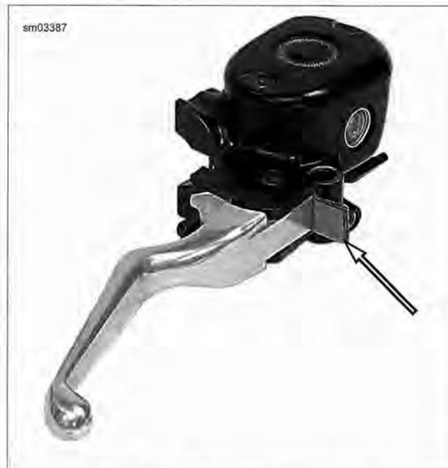
Figure 6-139. Install Cardboard Insert
