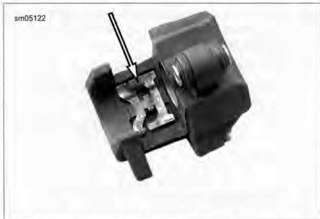
Figure 1-30. Rear Caliper Pad Spring
