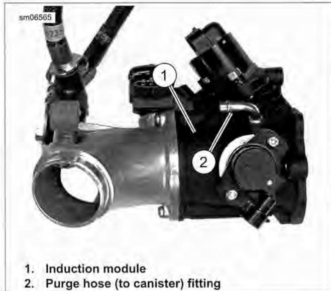
Figure 4-88. Emissions Hose Routing at Induction Module
