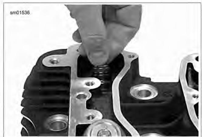
Figure 3-70. Valve Seal and Lower Valve Collar Assembly Installation
