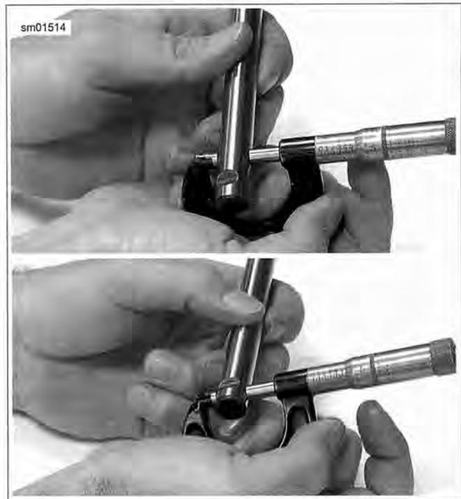
**Figure 3-53. Measuring Rocker Arm Shaft Diameter at Bushing Position (top) and Cover Position (bottom)**
