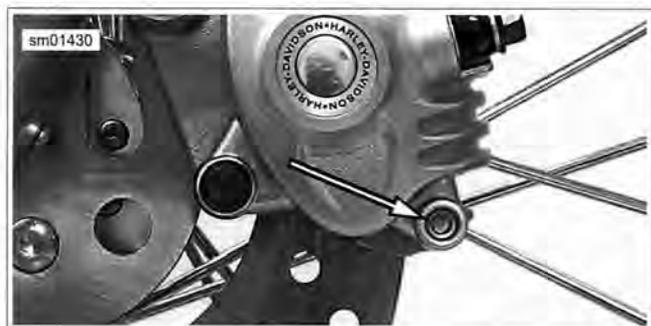
Figure 1-17. Brake Pad Pin (plug removed)
