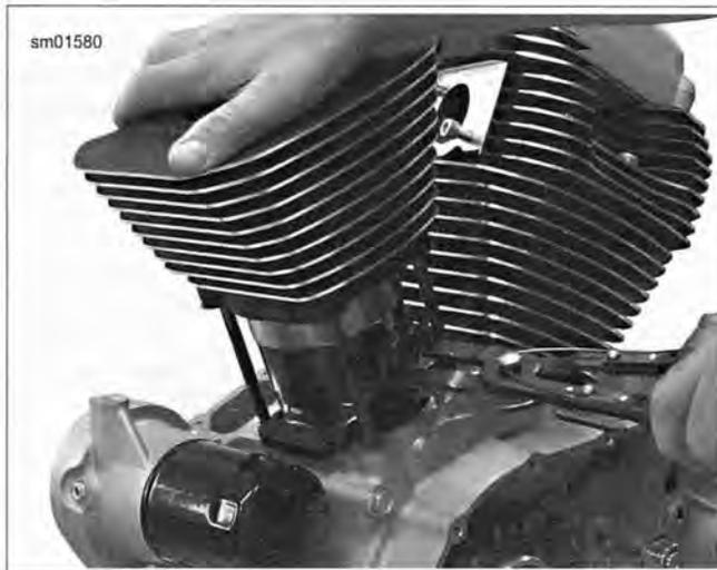
Figure 3-92. Installing Cylinder Over Piston
