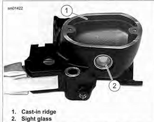
Figure 1-19. Filling Front Master Cylinder Reservoir (typical)
