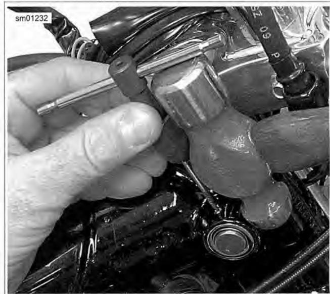
Figure 2-235. Removing Lock Pin
