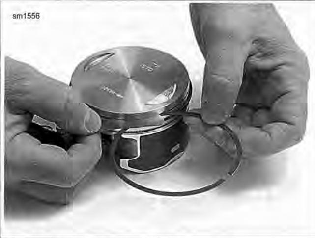
Figure 3-82. Measuring Ring Clearance in Groove (typical)
