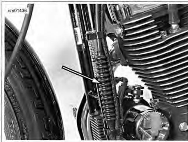
Figure 1-39. Clutch Cable Adjuster Location: XL Models
