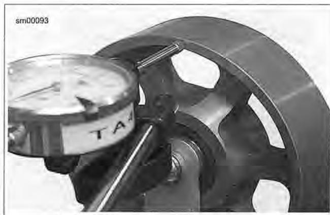
Figure 1-46. Measuring Lateral Side Play on Idler Pulley
