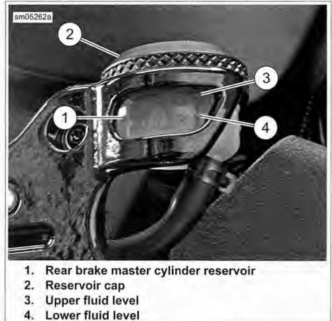
Figure 2-85. Rear Brake Master Cylinder Reservoir; XR 1200X
