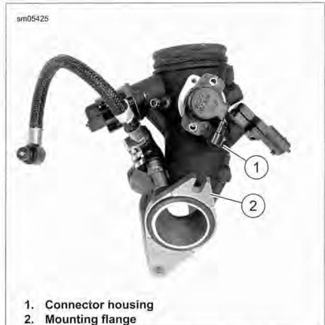
Figure 4-24. Throttle Position (TP) Sensor Installation: XR 1200X
