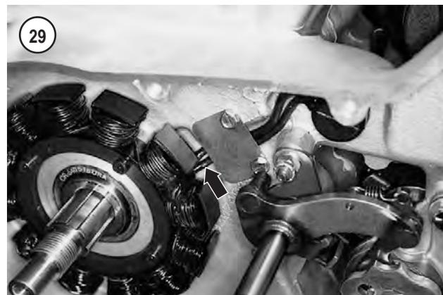
3. Do not operate the start switch if the ignition module is not grounded. The black ignition module wire is the ground wire. Inspect the wire end for corrosion and damage. Be sure the ignition module is mounted securely.
