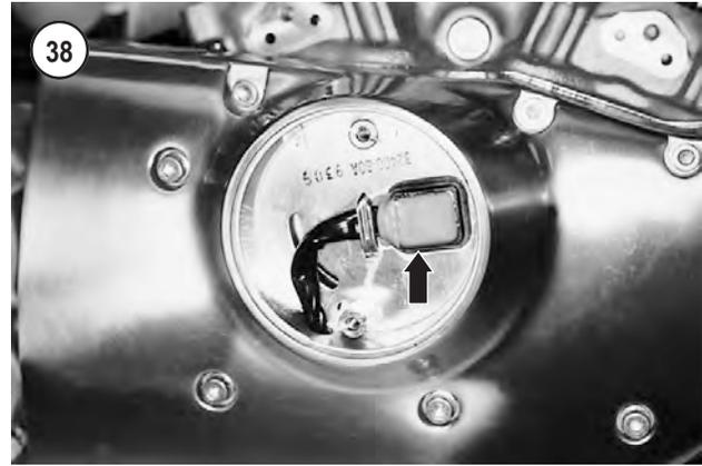
3. Spray the sensor (**Figure 38**) with a refrigerant (available at electronic supply stores). If the engine dies, replace the sensor as described in Chapter Twelve.
